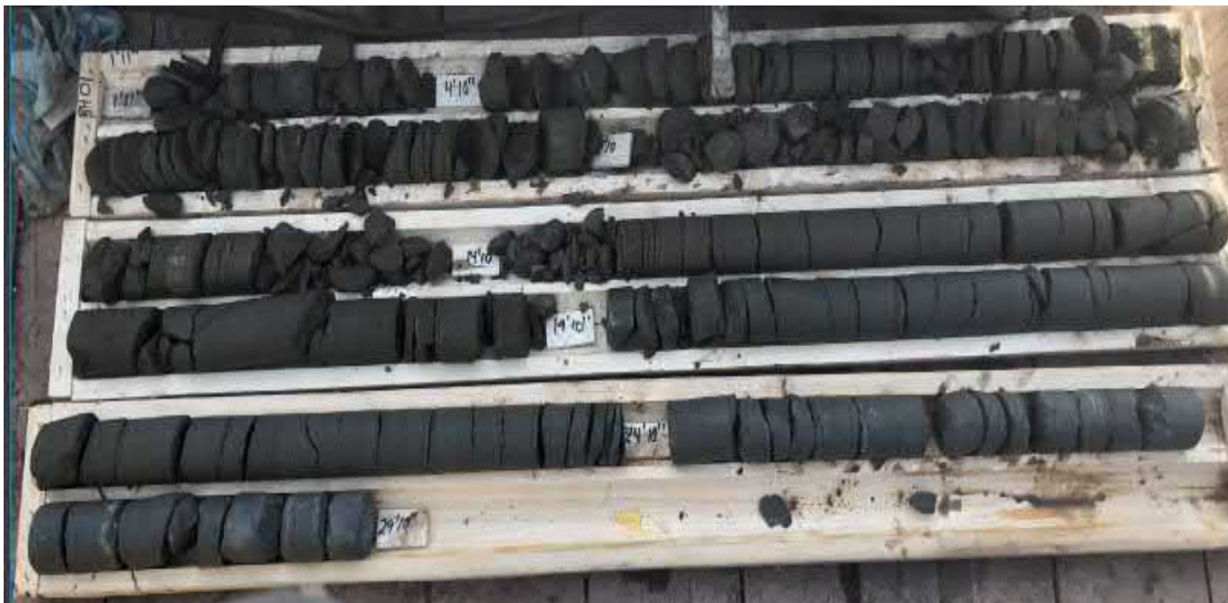
Photo 1: BH-18-01 Seabed Elevation : -1.7 meters Bedrock Elevation : -2.1 meters Amount cored : 8.6 meters
