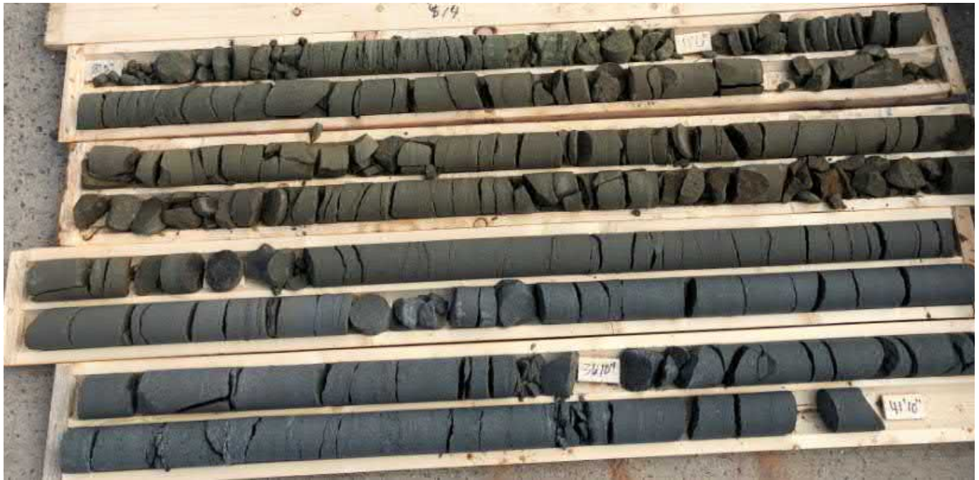
Photo 5: BH-18-05 Seabed Elevation :-1.2 meters Bedrock Elevation : -3.1 meters Amount cored : 10.9 meters
