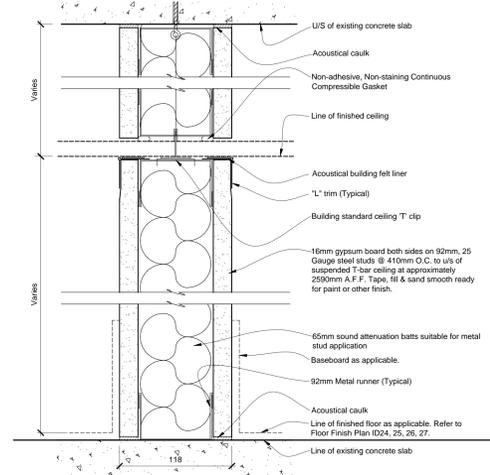
**1** Section - Interior Tenant Partition - Type 1 - U/S of Suspended T-bar Ceiling c/w Plenum Barrier
