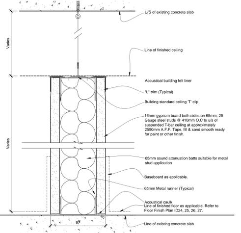
**3** Section - Interior Tenant Partition - Type 8 - U/S of Suspended T-bar Ceiling
