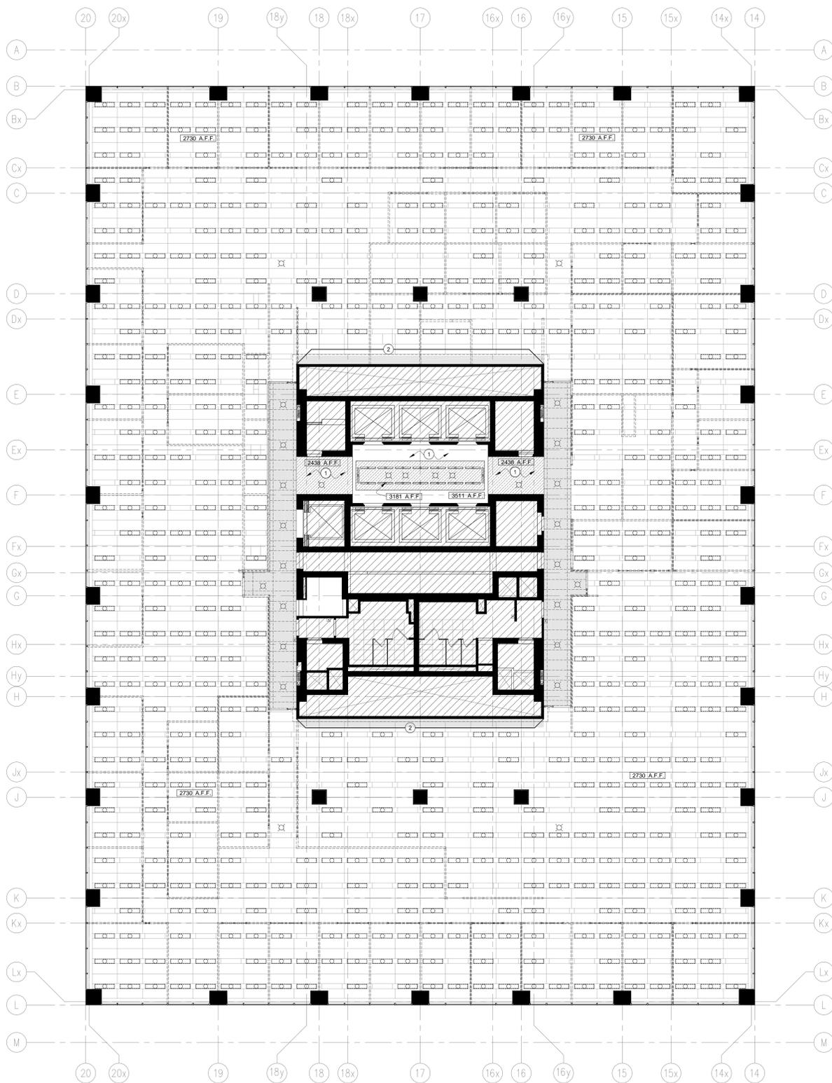
1 Reflected Ceiling Demolition Plan - 21st Floor
