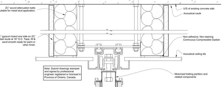
**8** Section - Plenum Barrier at Motorized Operable Partition
