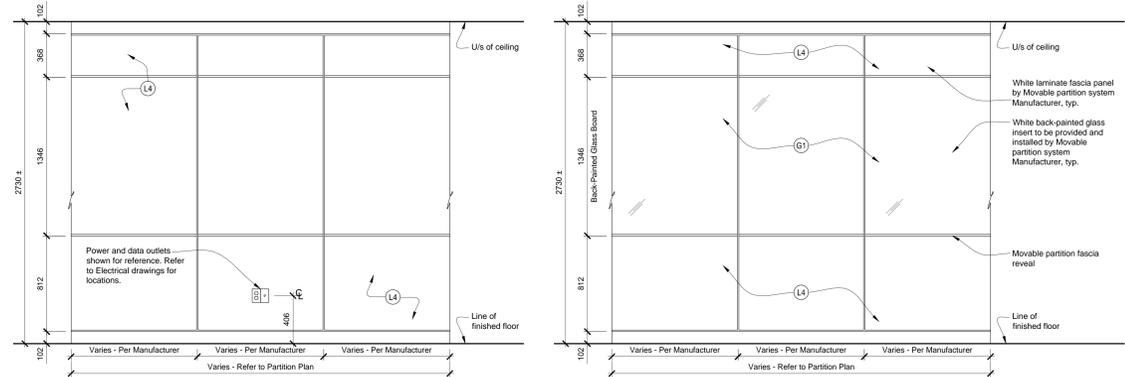
**5** Elevation - Typical Demountable Wall (Solid)
