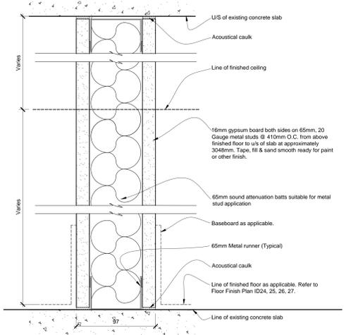
**2** Section - Interior Tenant Partition - Type 2 - Slab to Slab
