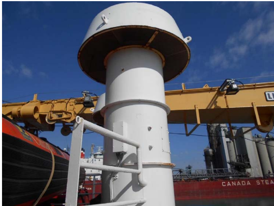
Figure 3: Photograph of in-situ ME supply axial fan.
