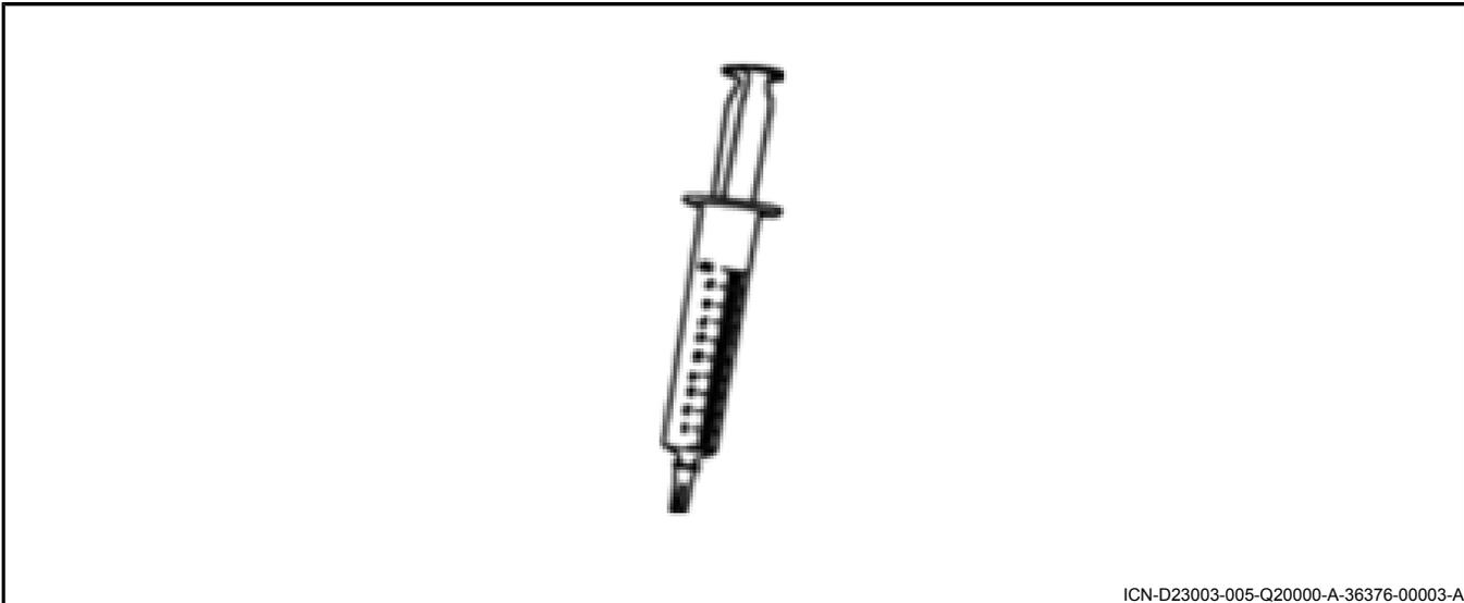
6. Insert syringe into patch through the spongy foam perimeter and inject 1.5 ml of the deionized water into the patch. With the syringe still in the patch, reposition the needle and evacuate any air in the patch. Once the air has been removed, inject the remaining 1.5 ml of water.
