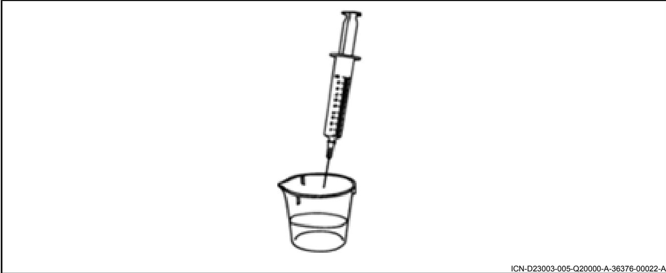
9. Measure the conductivity of the water using a digital conductivity meter.
