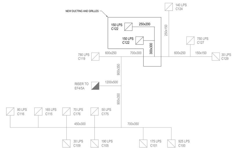
**SCHEMATIC - EXHAUST FAN E4/5A SYSTEM**
