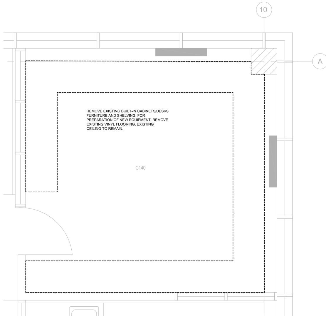
**PLAN (DEMOLITION) - LEVEL "C" - SECOND FLOOR, C140**
