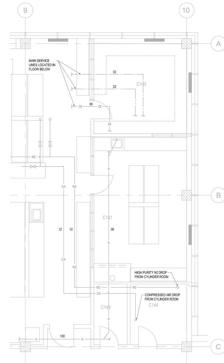
**PLAN (DEMOLITION) - LEVEL "C" - SECOND FLOOR, C140**
