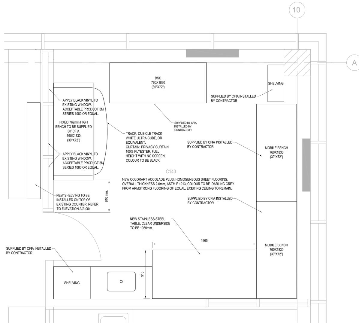
**PLAN (NEW CONSTRUCTION) - LEVEL "C" - SECOND FLOOR, C140**
