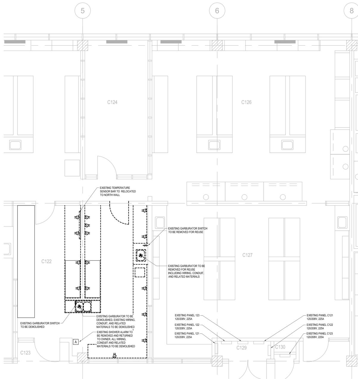
**PLAN (DEMOLITION) - LEVEL "C" - SECOND FLOOR, C122 & C126**
