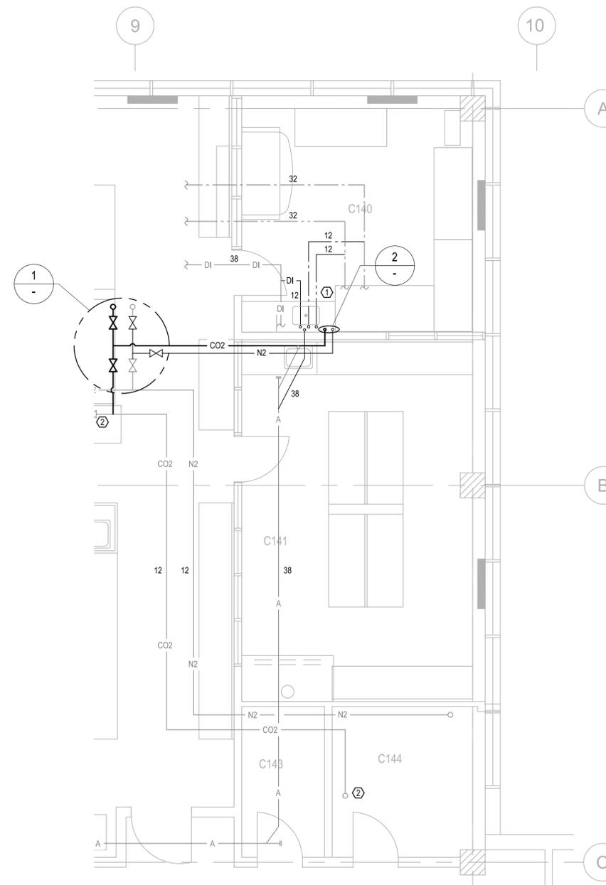
**PLAN (NEW CONSTRUCTION) - LEVEL "C" - SECOND FLOOR, C140**
