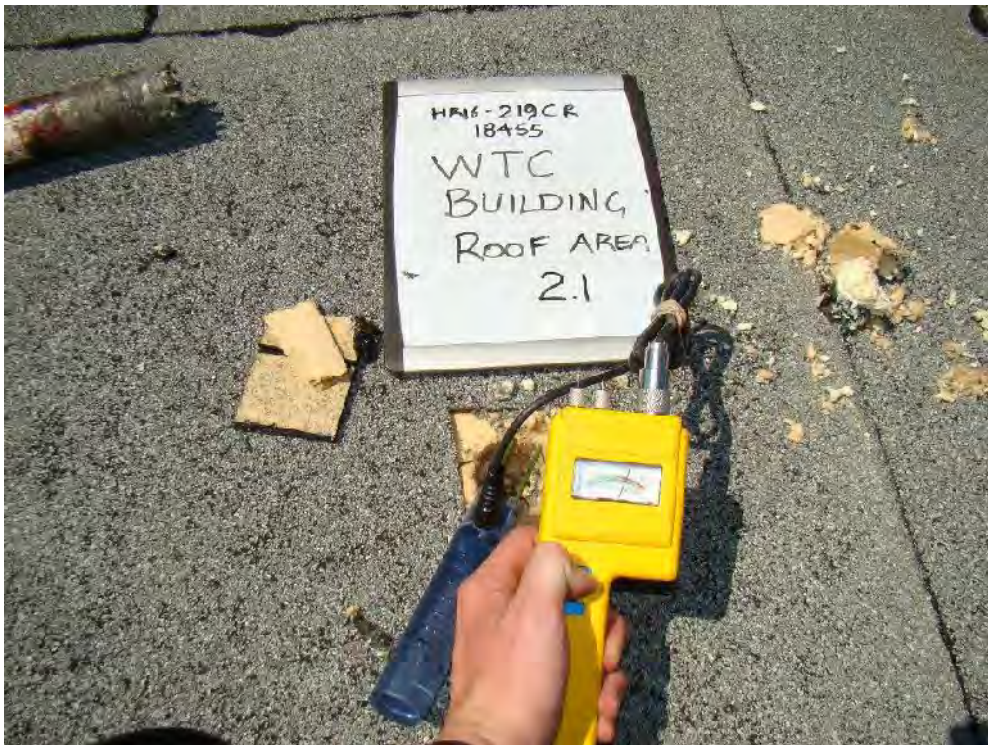
Photograph 56: Roof Area 2.1 Test Cut – High moisture levels were detected within the top layer of fibreboard insulation.
