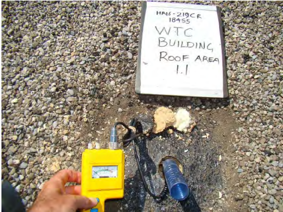
Photograph 5: Roof Area 1.1 Cut Test – The membrane at the core cut location appeared well bonded to the fibreboard substrate and adhesion between membrane layers was noted to be good. Probes taken at the core cut location revealed no moisture present in the insulation layer or within the membrane interply.
