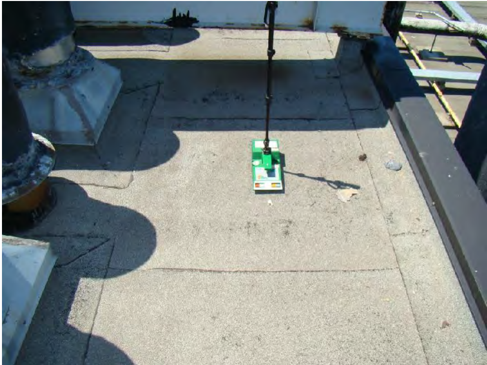
Photograph 69: Roof Area 3.1 – Testing with the Tramex Moisture Detection Instrument detected moisture contamination of the underlying insulation components throughout the entirety of the roof. The entire roof was noticeably “soft” under foot indicative of insulation which is saturated.
