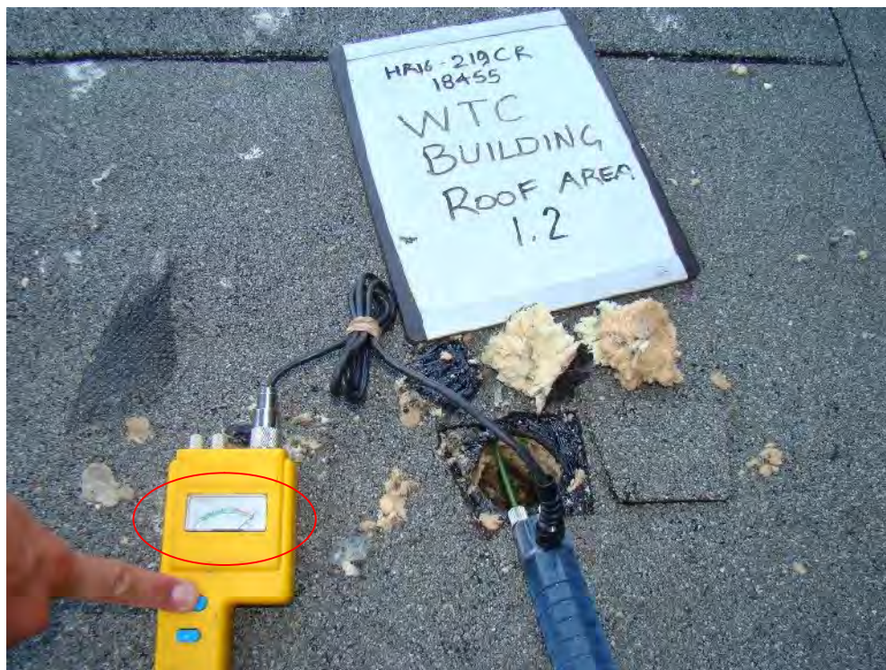
Photograph 30: Roof Area 1.2 – Test Cut #1 - Probes confirmed high readings of “70” to “95” within the thermal insulation layers below the membrane. All insulation layers at this location were visibly wet and moisture damaged. It was noted that an additional layer of tapered insulation was present at this first core test location in order to provide back slope away from the wall.
