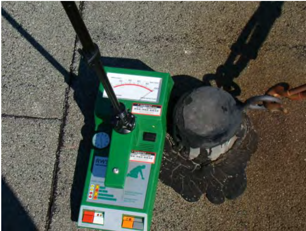
Photograph 23: Roof Area 1.2 – Moisture detected adjacent to guy wire pitch pocket penetrations.
