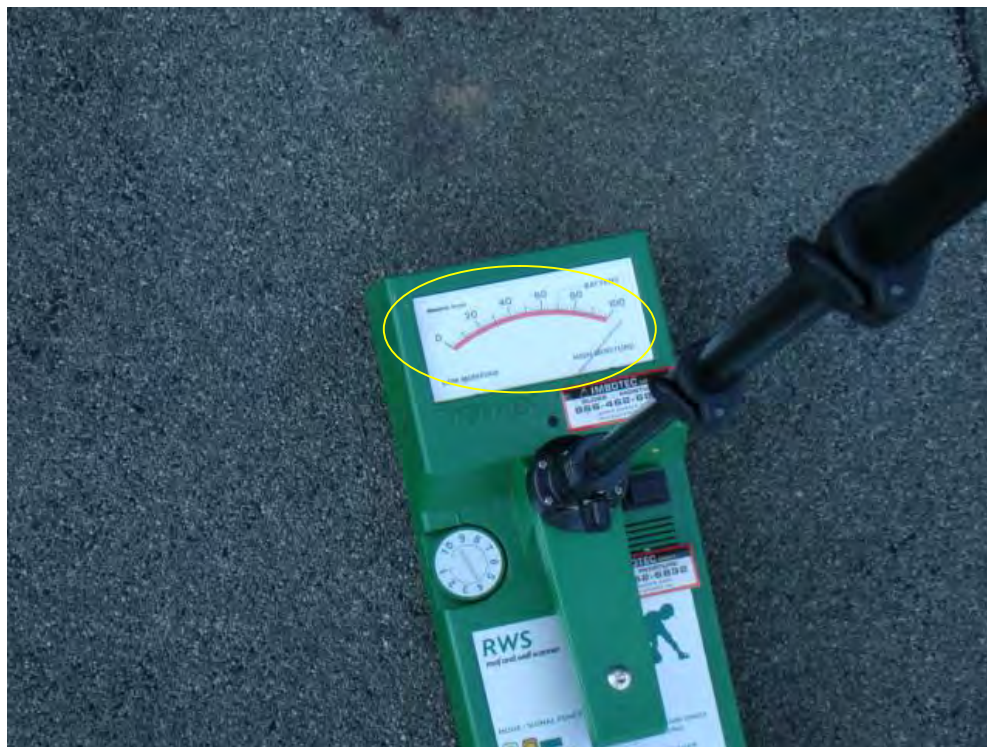
Photograph 22: Roof Area 1.2 – Closer view showing high moisture readings at location shown in previous photo.
