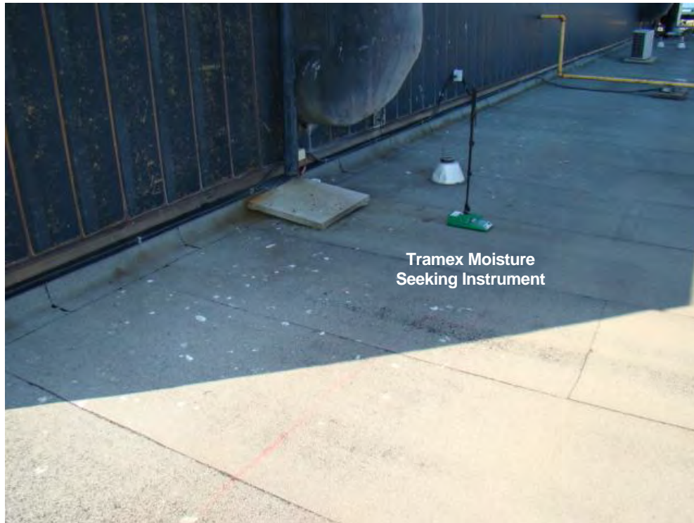
Photograph 21: Roof Area 1.2 – Moisture detected along the north penthouse wall.
