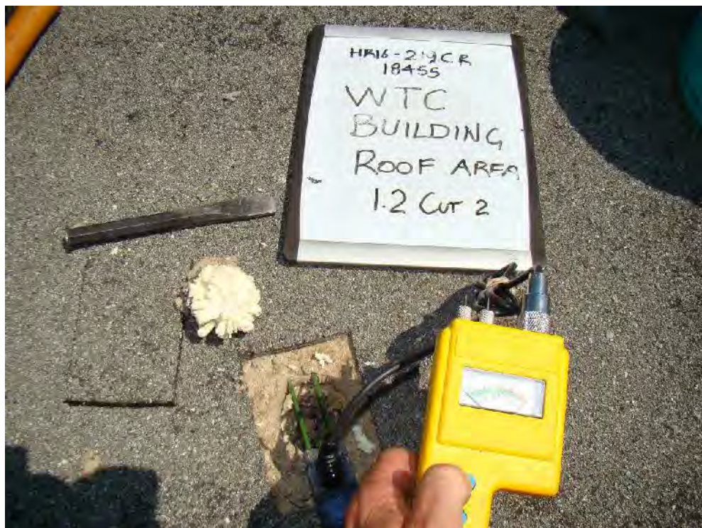
Photograph 32: Roof Area 1.2 – Test Cut #2 - Probes taken at this location revealed no moisture present in the insulation layer or within the membrane interply.
