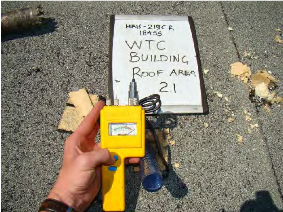
Photograph 55: Roof Area 2.1 Test Cut – High moisture levels were detected within the base layer of polyisocyanurate insulation.
