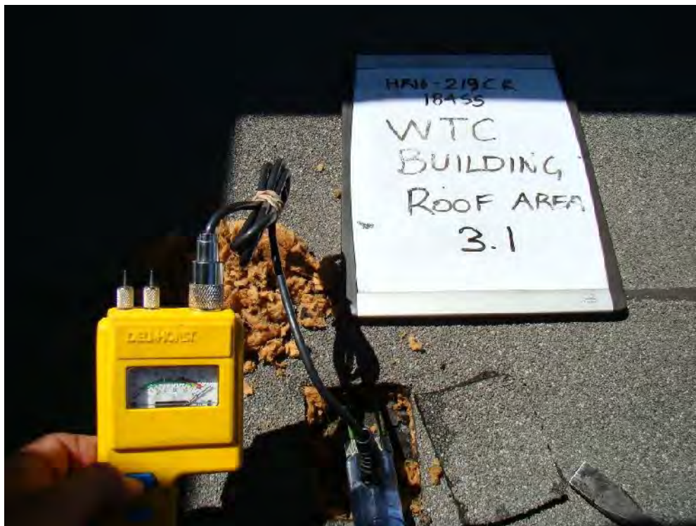
Photograph 72: Roof Area 3.1 Test Cut – Probes showed significant moisture readings of “100” within the insulation. Both the base layer of polyisocyanurate insulation and fiberboard layer were found to be saturated. The only component preventing widespread leakage is the presence of a sound 2 ply felt vapour retarder applied to the gypsum board substrate secured to the steel deck.
