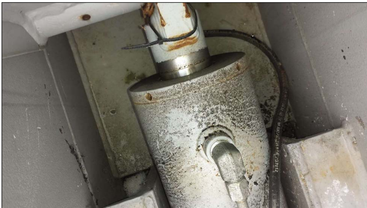
Figure 13 - Partial view of one of the extension cylinders inside boom. Photo: Garage PEM Barrette 2015.
