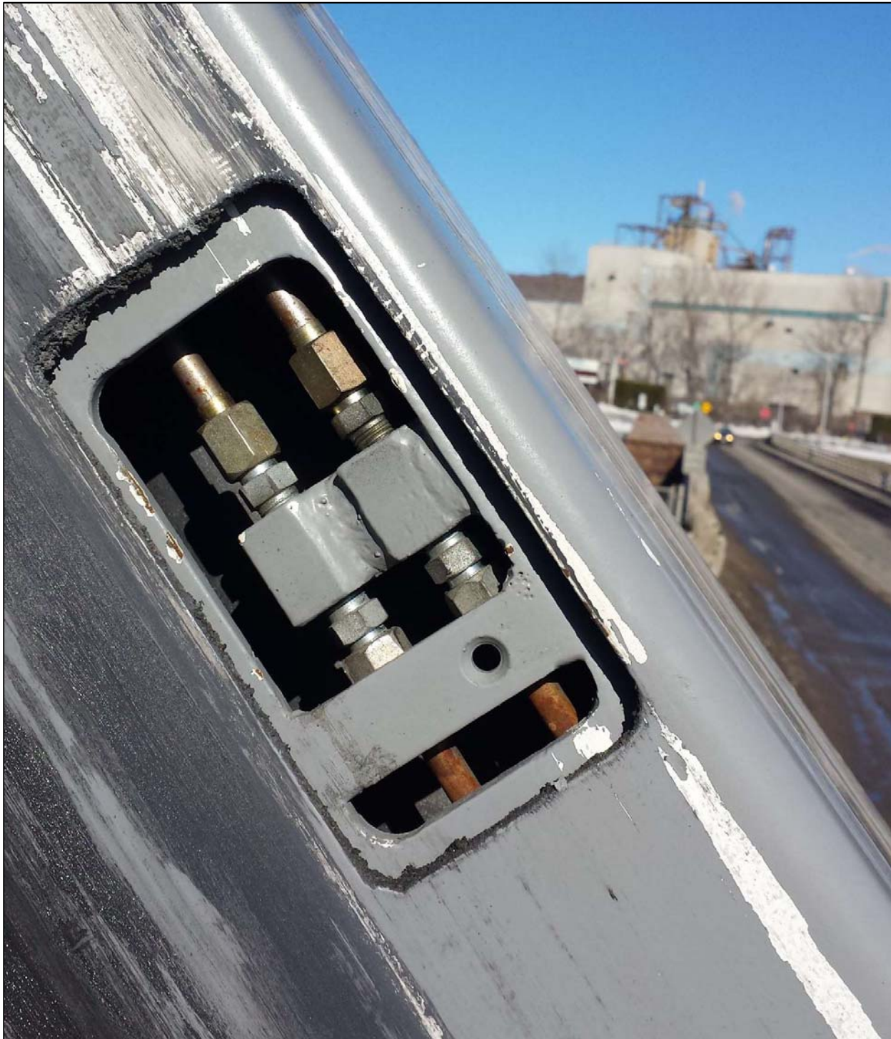
Figure 16 - Hydraulic connections inside boom. Photo: Garage PEM Barrette, 2015.
