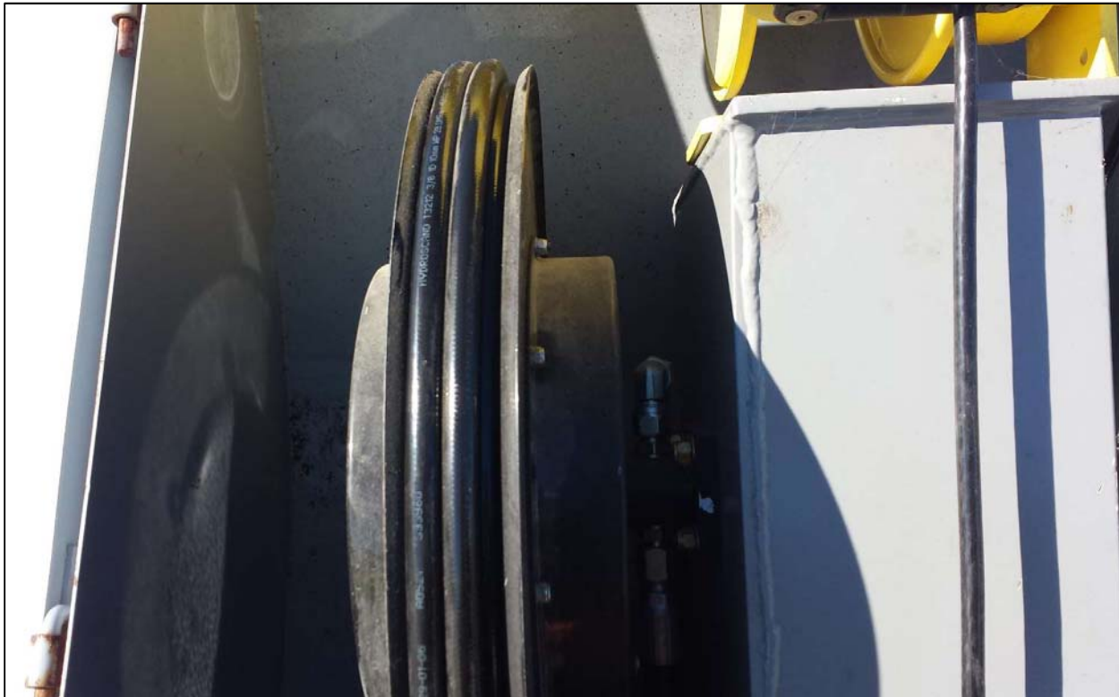
Figure 15 - Hydraulic hose reel on top of boom. Electric cable reel at top right corner of photo. Valves at centre of picture. Photo: Garage PEM Barrette, 2015.
