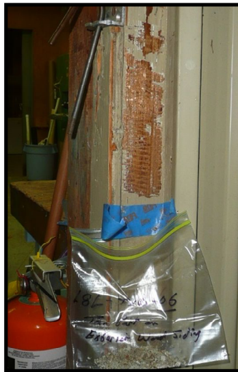
Tan Paint Sample 18L-TSB-06 from the exterior side of the wood siding (Original Cladding) at the east entrance
