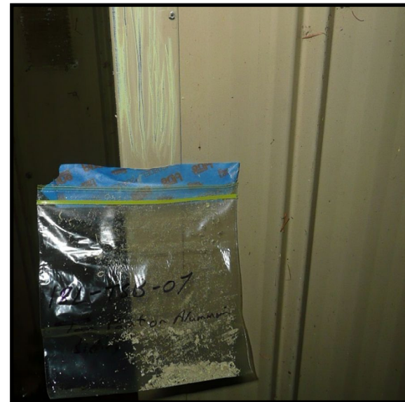
Tan Paint Sample 18L-TSB-07 from the exterior metal siding (Newer Cladding) of the buildings' northeast corner.
