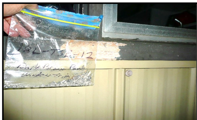
Dark Brown Paint Sample 18L-TSB-12 from the exterior side of wooden window frame at Paint Shop # 6 and Office #3.
