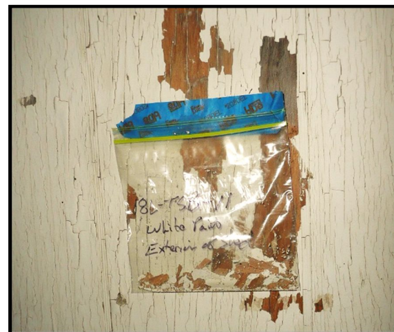
White Paint Sample 18L-TSB-11 and Painted Base Substrate TCLP Sample 18TCLP-TSB-11 from the wood exterior siding of the storage shed.
