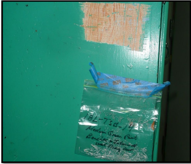
Medium Green Paint Sample 18L-TSB-14 and Painted Base Substrate TCLP Sample 18TCLP-TSB-14 from the Machine Shop benches and interior side of exit door.
