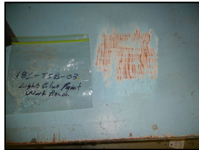
Light Blue Paint Sample 18L-TSB-03 and Painted Base Substrate TCLP Sample 18TCLP-TSB-03 from the wooden work bench in the Carpenters Shop Room # 7.
