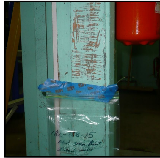
Mint Green Paint Sample 18L-TSB-15 from the Machine Shop interior walls.
