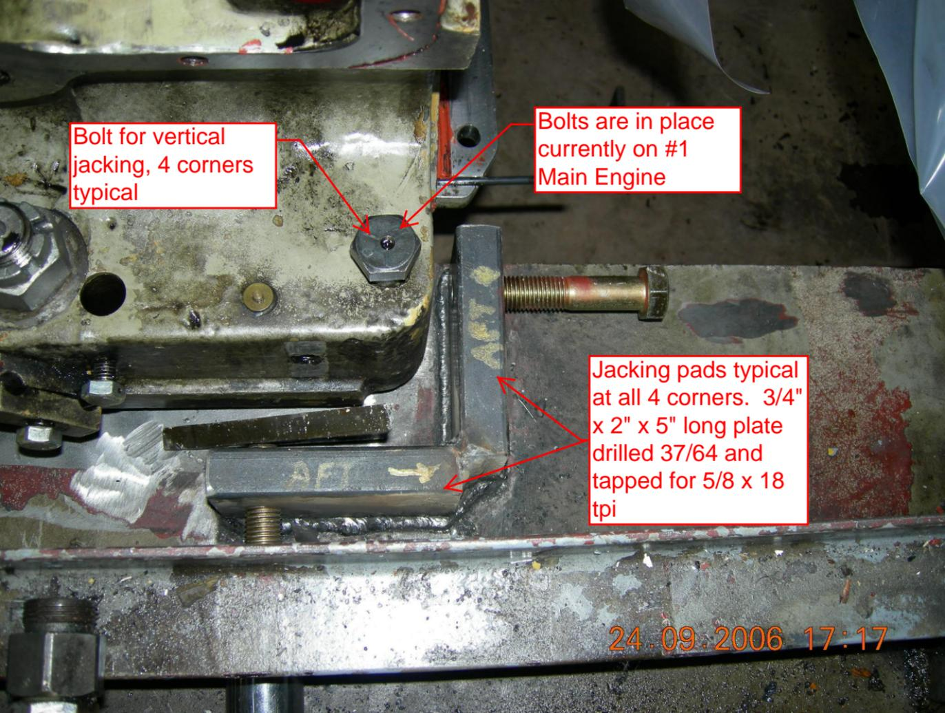
Bolt for vertical jacking, 4 corners typical
