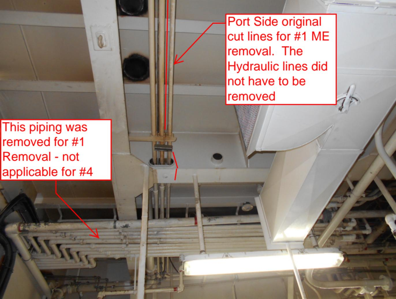
Port Side original cut lines for #1 ME removal. The Hydraulic lines did not have to be removed
