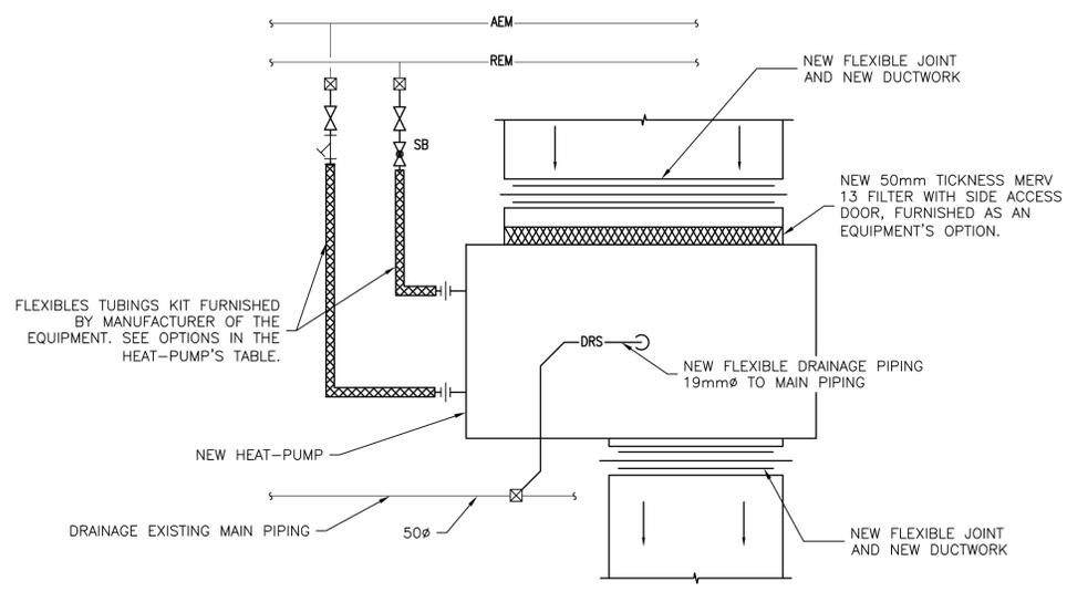
**TYPICAL DETAIL – INSTALLATION OF A HEAT-PUMP (REPLACEMENT)**
