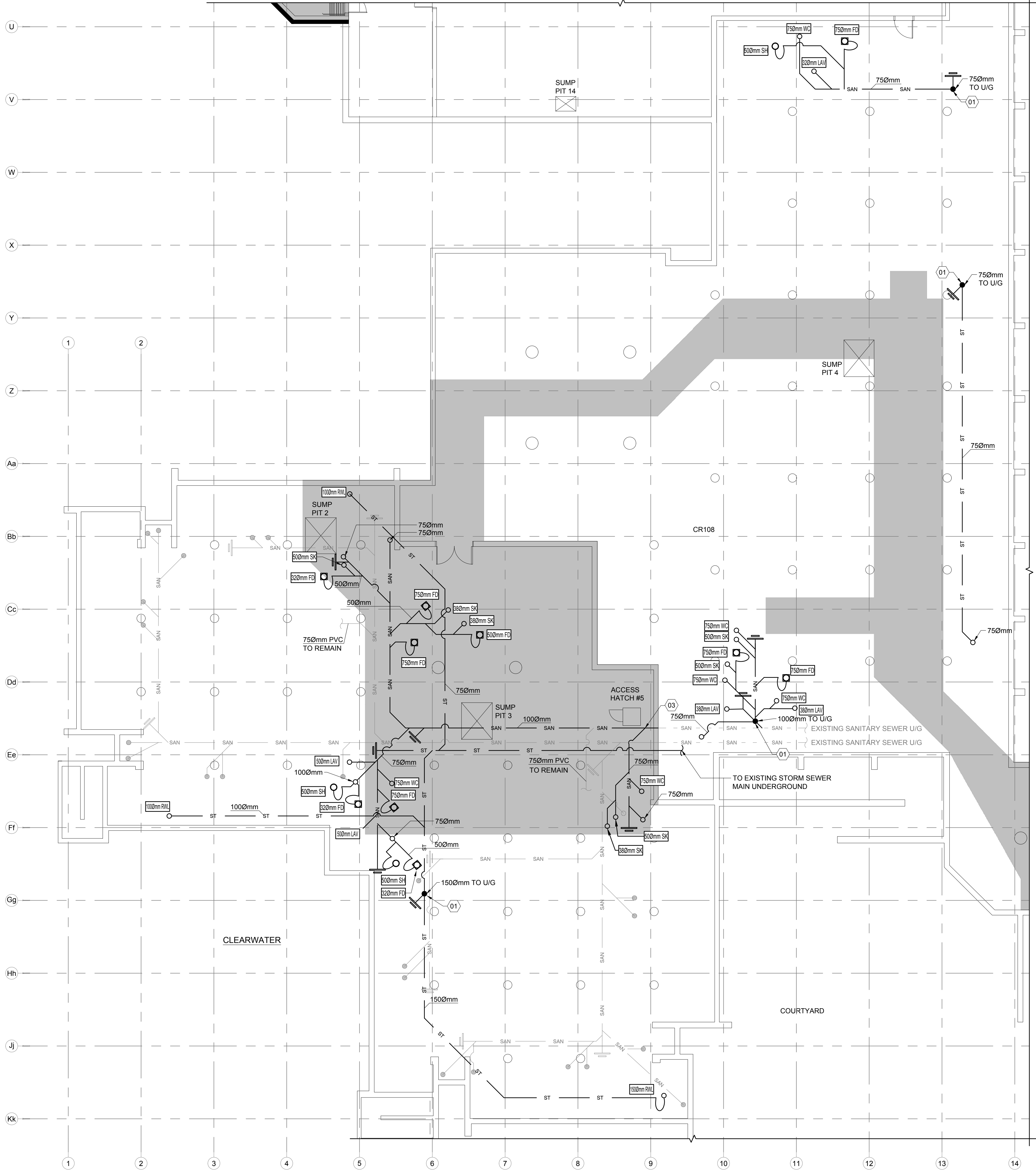
1 M101 CLEARWATER PIPING CONSTRUCTION PLAN - PARTIAL
