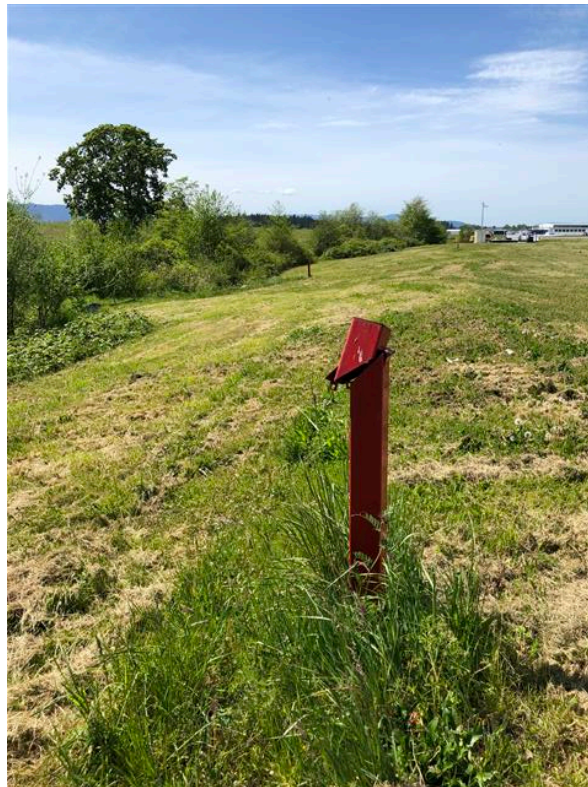
Photo 12: Monitoring wells adjacent to Reach 1A and Reach 1C to be protected.
