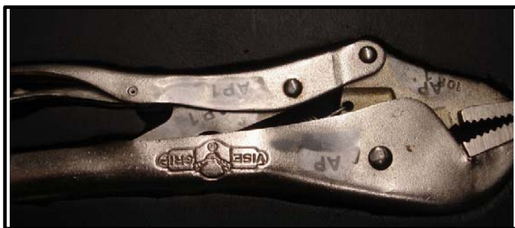
Photo 5 All removable parts which could be removed/loosened from its owner tool, will be etched. This photo is an example of the concept.
