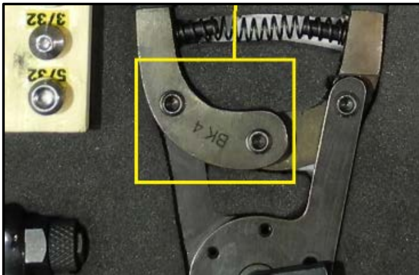
Photo 4 Present etching method – new method will have number as per annex B
