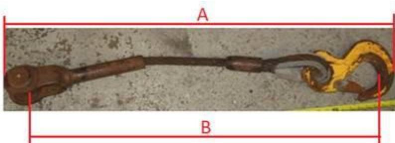
1 meter is stated as the overall length, are you measuring bearing point to bearing point? Length B is Bearing Point to Bearing point, which is standard measuring length in the industry. We need to know how the assembly was measured to get the proper length, as there is no tape measure in the picture.
