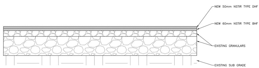
ASPHALT SURFACE RESTORATION DETAIL (1) C03/C06
