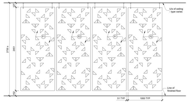
1 Elevation - Typical Felt Dividers
