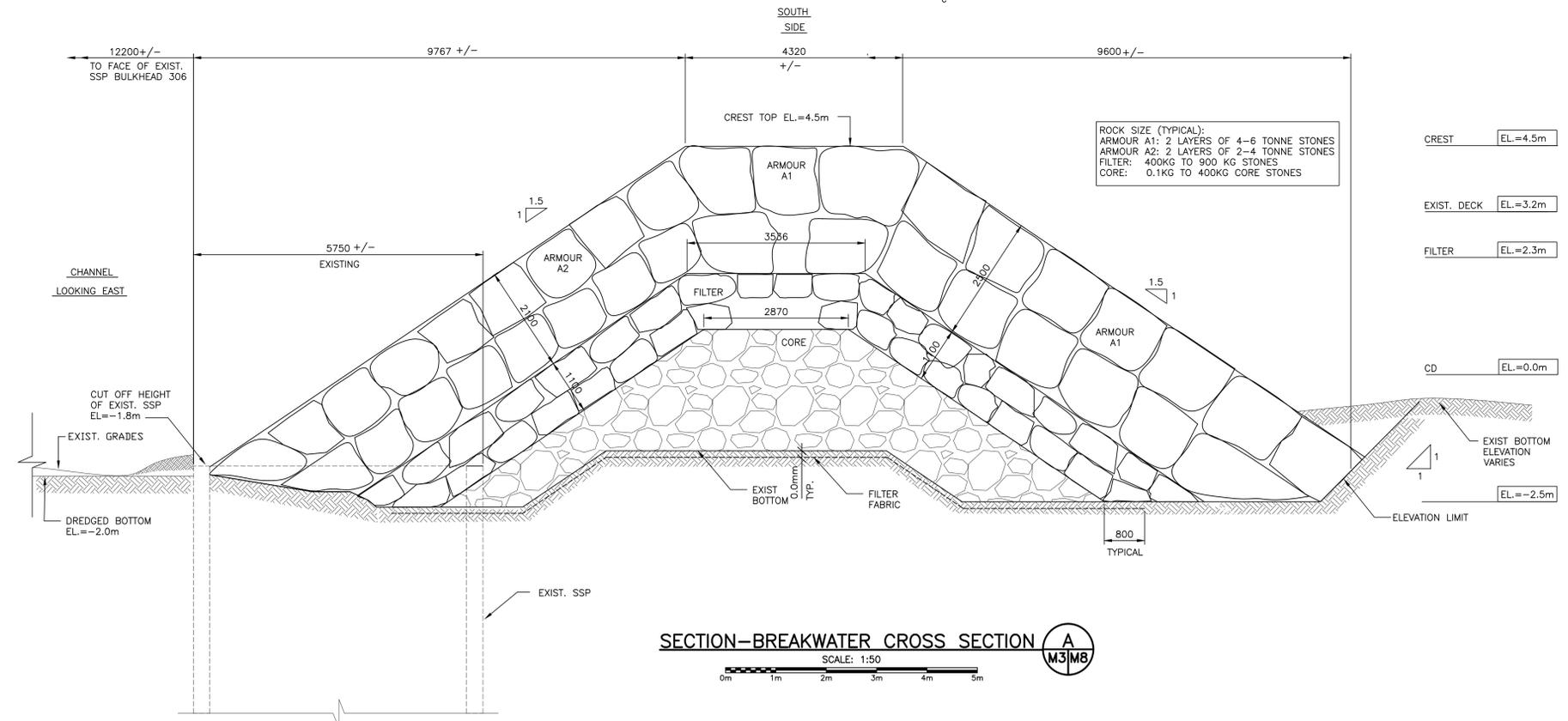
**SECTION-BREAKWATER CROSS SECTION A**
