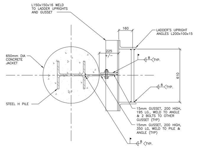
**SECTION-LADDER CONNECTION TO PILE** B
