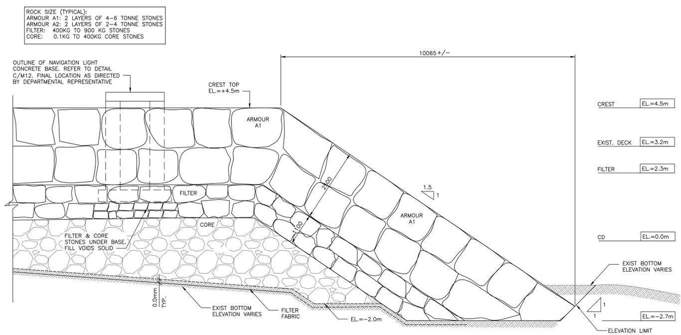
**SECTION-BREAKWATER CROSS SECTION B**
