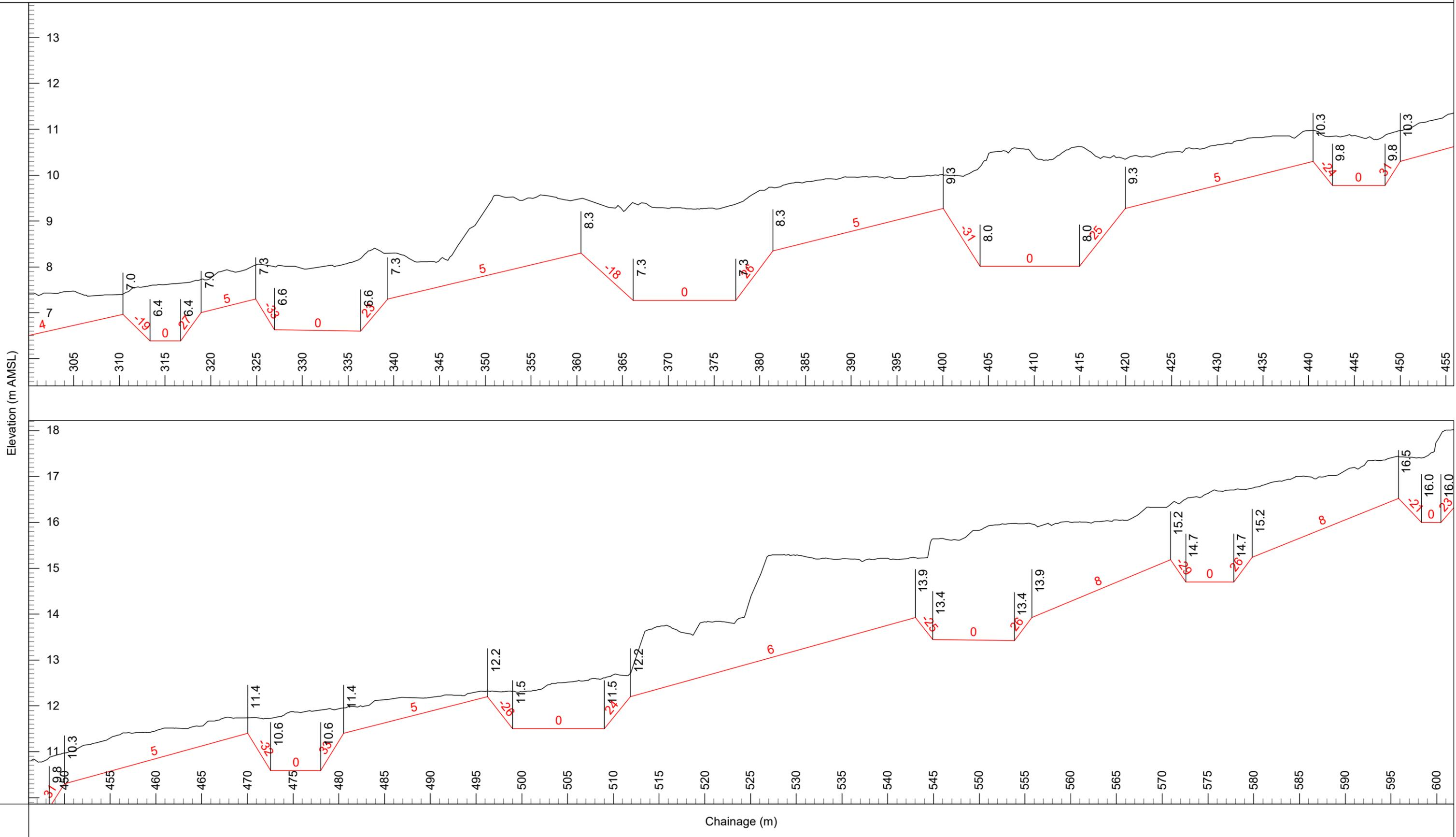
Note: Profiles were generated from digital elevation model derived from LiDAR data.
