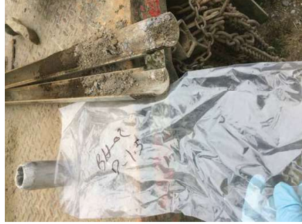
Photo 6 - BH-02 - Sand D-1.50 m
