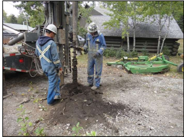
Photos 01 and 02: Drilling TH-1 east of the log building.
