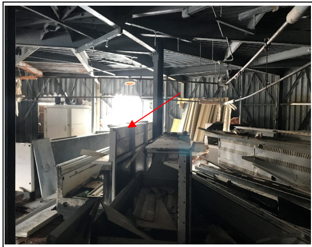
Photo 12: Building 1A – Suspect ODS-containing refrigerator display units.
