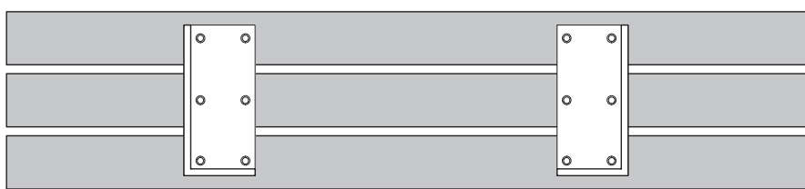
REFLECTED PLAN E-E: Fixings viewed from below
