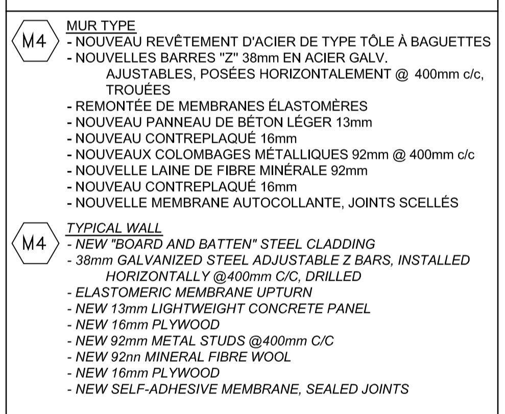
COMPOSITIONS TYPES TYPICAL COMPOSITIONS M4 TYPICAL WALL - NEW "BOARD AND BATTEN" STEEL CLADDING - 38mm GALVANIZED STEEL ADJUSTABLE Z BARS, INSTALLED HORIZONTALLY @ 400mm C/C, DRILLED - ELASTOMERIC MEMBRANE UPTURN - NEW 13mm LIGHTWEIGHT CONCRETE PANEL - NEW 16mm PLYWOOD - NEW 92mm METAL STUDS @ 400mm C/C - NEW MINERAL FIBRE WOOL - NEW SELF-ADHESIVE VAPOUR BARRIER, SEALED JOINTS - EXTERIOR GYPSUM BOARD TO BE KEPT - EXISTING STEEL DECKING TO BE KEPT
