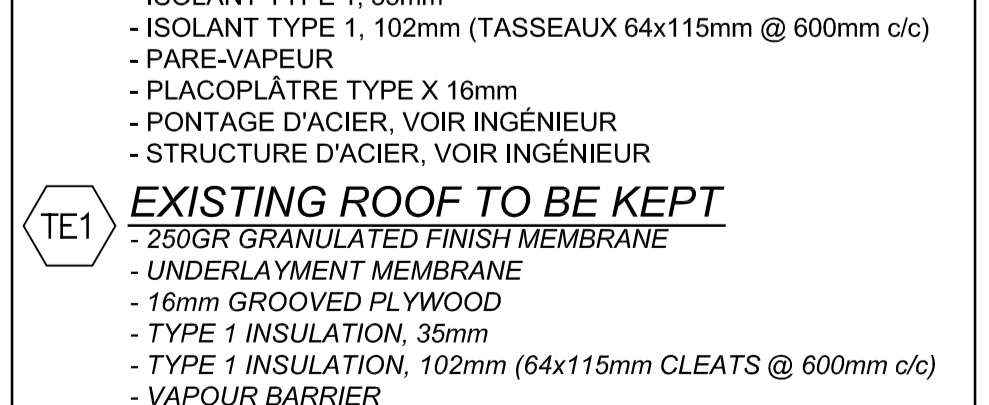
COMPOSITIONS TYPES TYPICAL COMPOSITIONS TE1 EXISTING ROOF TO BE KEPT - 250GR GRANULATED FINISH MEMBRANE - UNDERLAYMENT MEMBRANE - 16mm GROOVED PLYWOOD - TYPE 1 INSULATION, 35mm - TYPE 1 INSULATION, 102mm (64x115mm CLEATS @ 600mm c/c) - VAPOUR BARRIER - 16mm TYPE X GYPSUM BOARD - STEEL DECKING, SEE ENG. - STEEL STRUCTURE, SEE ENG.
