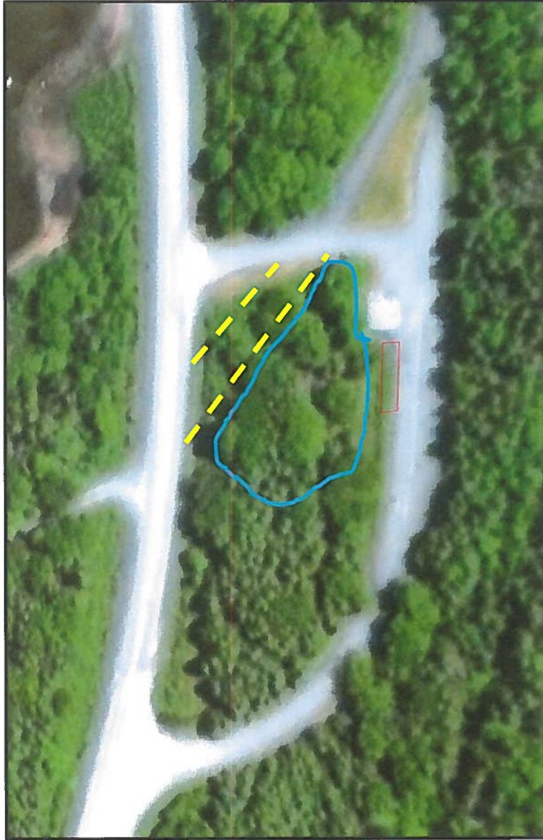
Figure 5. Google Earth image - Yellow dotted lines indicate former highway, probably disturbed with leveling and fill activities during original construction. The blue line represent a wet area which is potentially the result of poor drainage in the area, as indicated by the Resource Management Officer. At the time this report was written, the culverts had recently been unclogged in a nearby area. Overall, the area seems to be, have been disturbed by surrounding roadways and Kiosk footprint (Rod Cox: Pers. Com. 2016).
