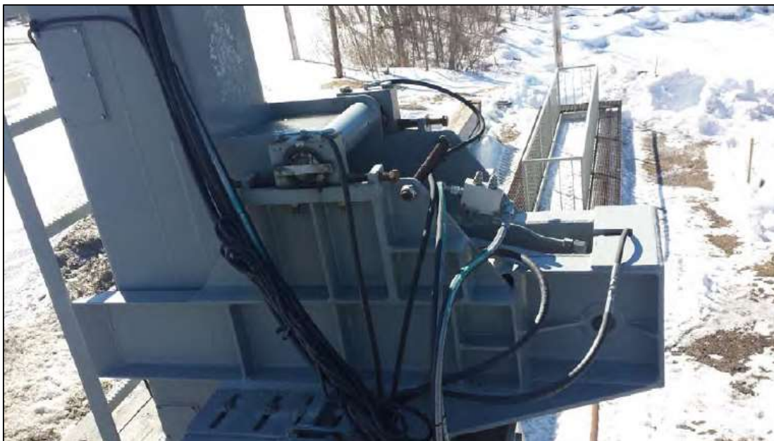
Figure 8 - Connection between boom and frame of stoplog lifter. Photo: Garage PEM Barrette, 2015.
