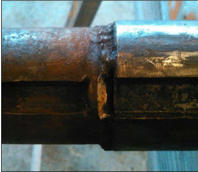
Figure 14 - Contrary to the as-built drawings, the Quebec shaft contained a weld. There was no visible crack, but the phased-array ultrasonic test had detected one, and this shaft was replaced with a new fabrication.
