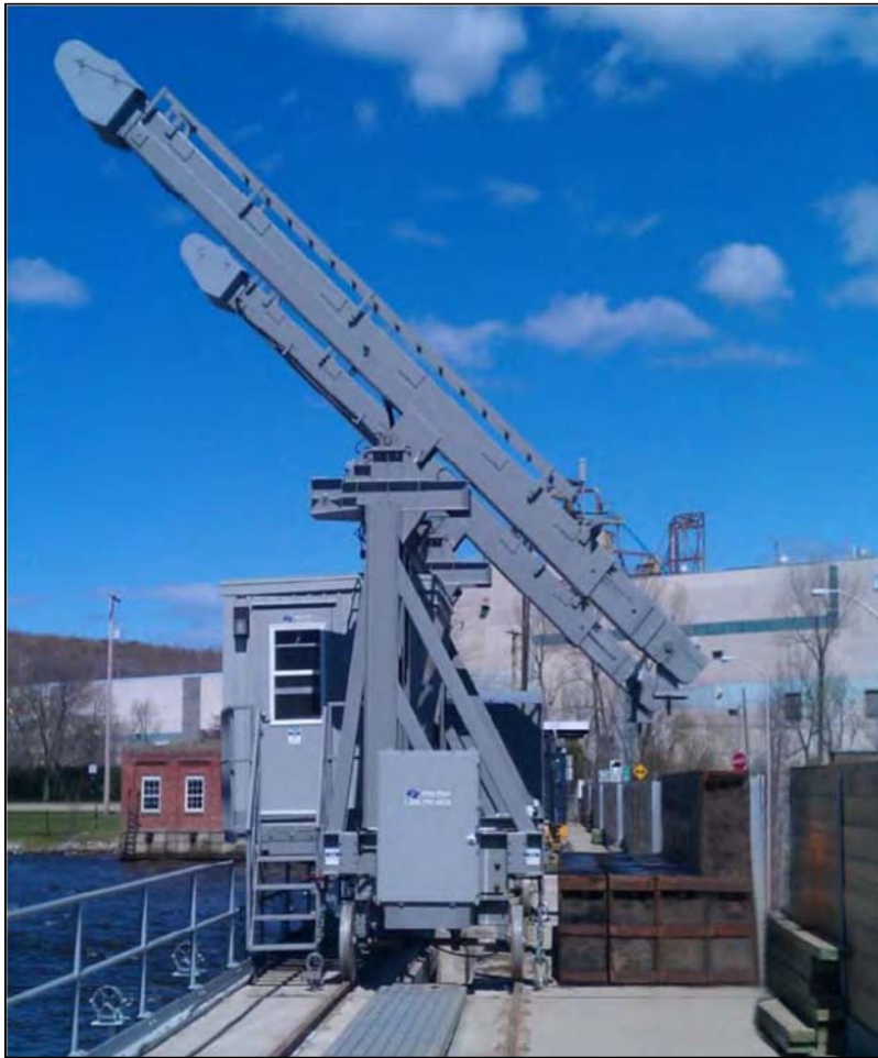
Figure 7 - Quebec stoplog lifter.
