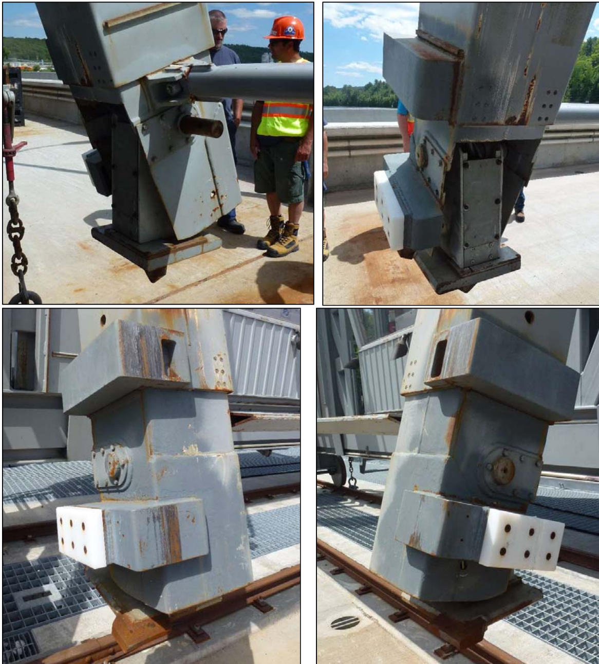
Figure 11 - Four views of end of a boom on the Ontario stoplog lifter, showing guide pieces added to accommodate the newly-widened sluices on the new Ontario dam.
