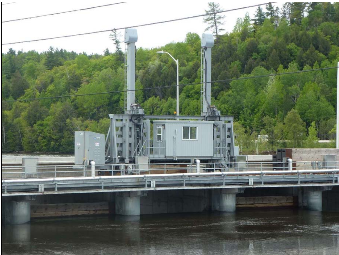
Figure 3 - Ontario stoplog lifter, upstream side.
