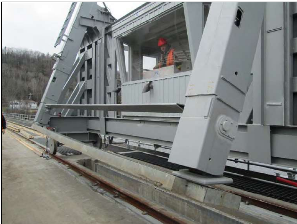
Figure 5 - Ontario stoplog lifter (before modifications) manipulating a cover from the top of a sluice.
