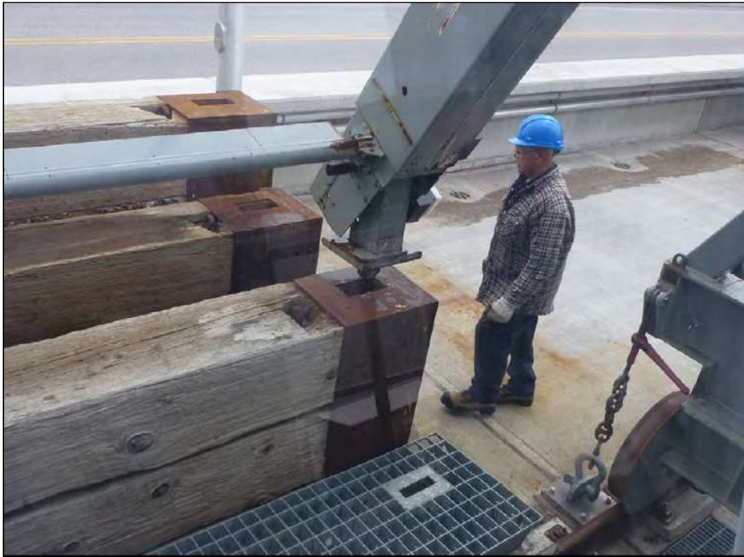
Figure 6 - Ontario stoplog lifter (after installation of guide pieces) getting ready to pick up a double-stoplog from the deck.
