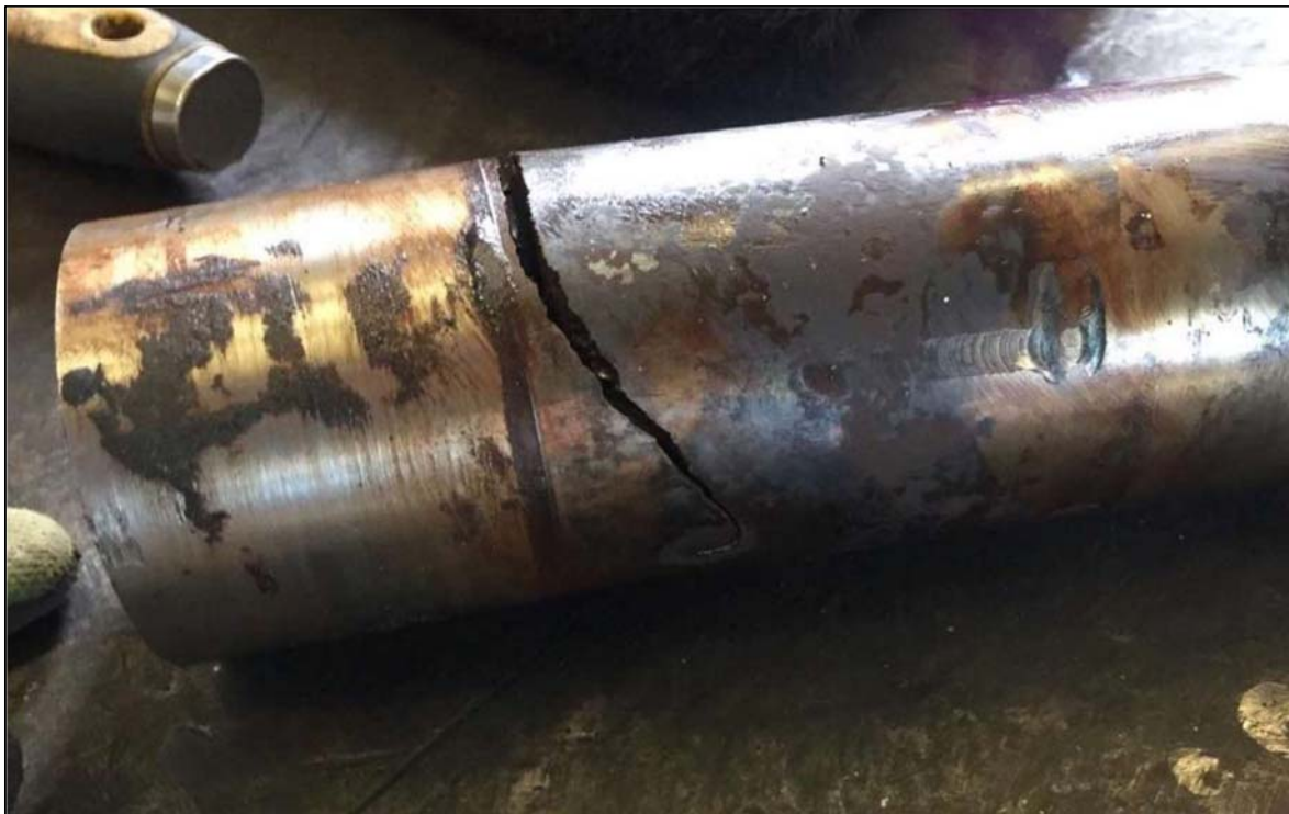
Figure 13 - Ontario stoplog lifter's broken axle.
