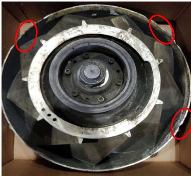
Figure 1 and 2 – Typical damages to the casing, fins and splines
