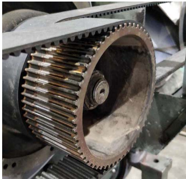
Figure 1 and 2 – Typical damages to the casing, fins and splines
