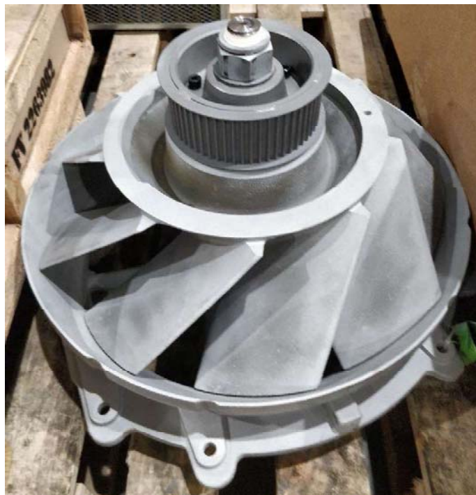
Figure 3 – Refurbished cooling fan
