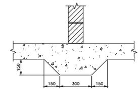
**TYP. EXIST. THICKENED SLAB DETAIL**
