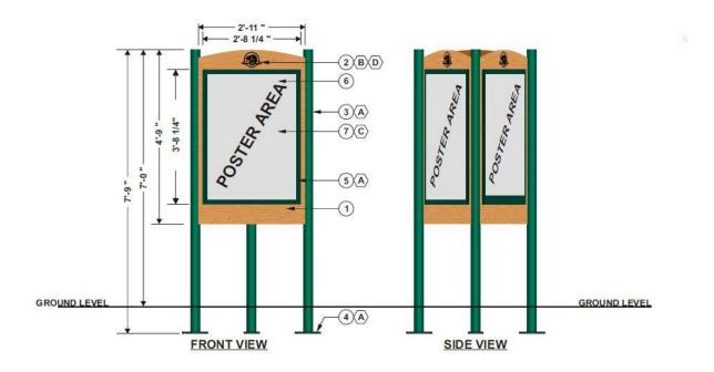
**Pylon Posters Specifications:** Fabricated using a clear-non glare polycarbonate face, digitally printed on second surface, using vinyl applied to print on second surface. Polycarbonate is <u>a recyclable material</u> with minimal impact on the environment.
