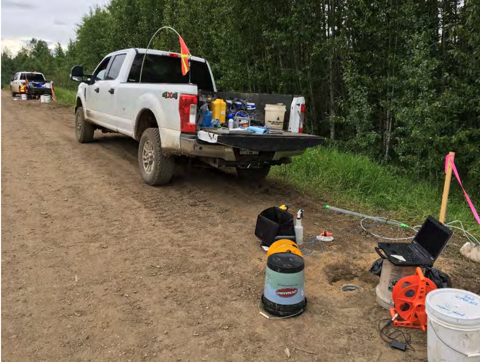
Photo 9: Slug testing at K19-MW17-29D AEC 1b
