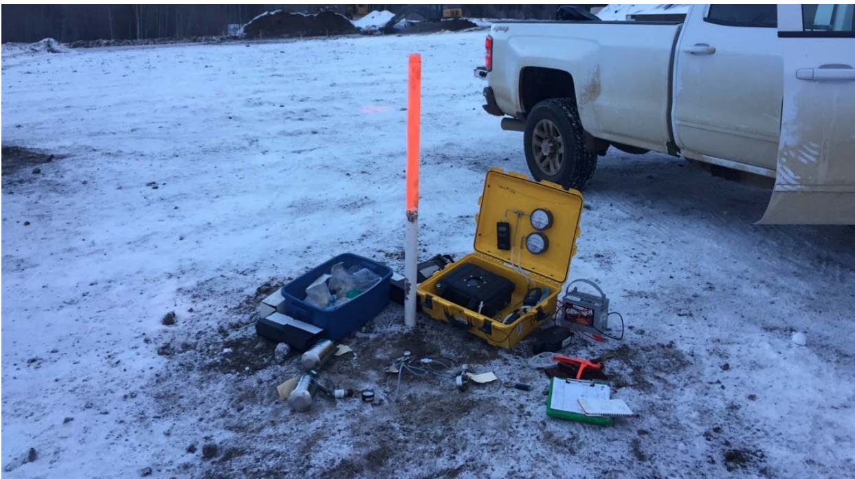
Photograph 10: Soil vapour sampling at K19-SV18-03. 19 January 2018.
