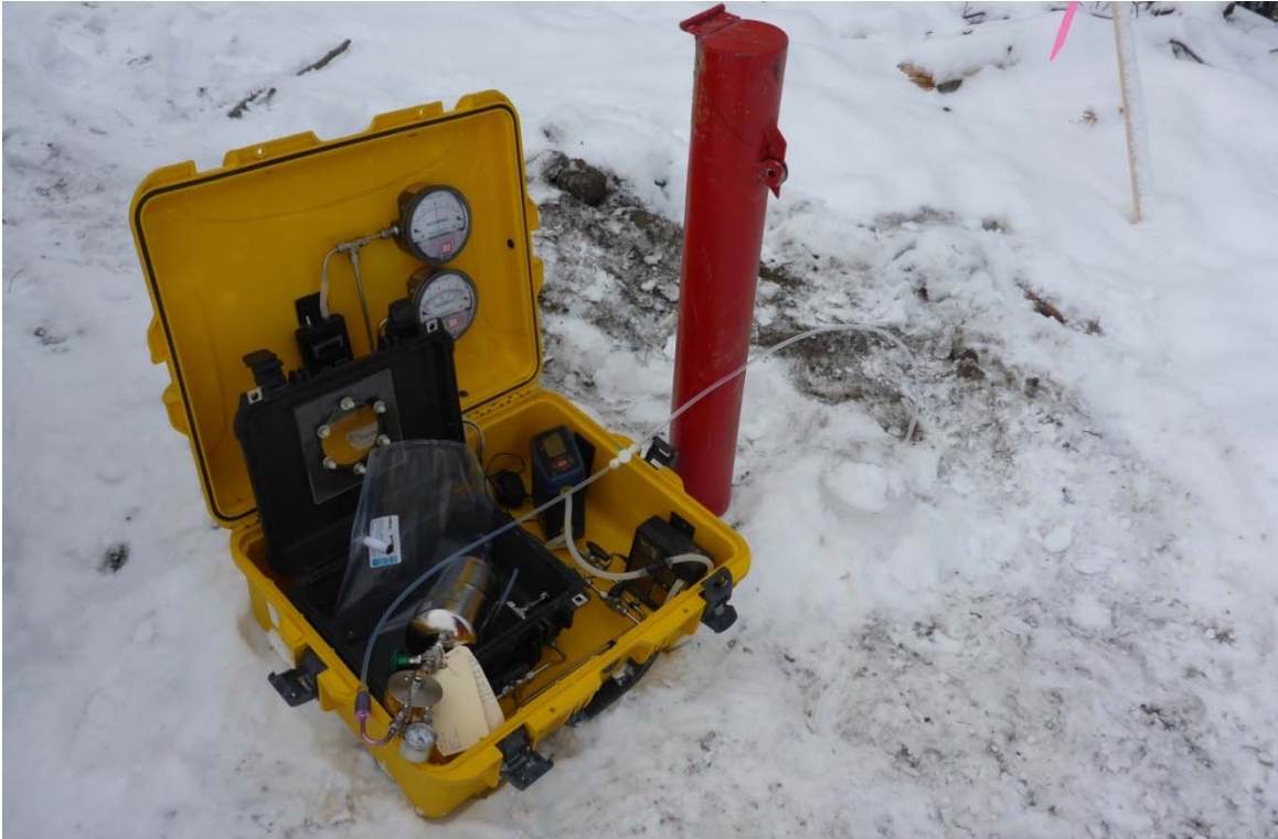
Photograph 11: Soil vapour sampling at K19-SV18-06. 22 January 2018.
