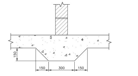
**TYP. EXIST. THICKENED SLAB DETAIL K**
