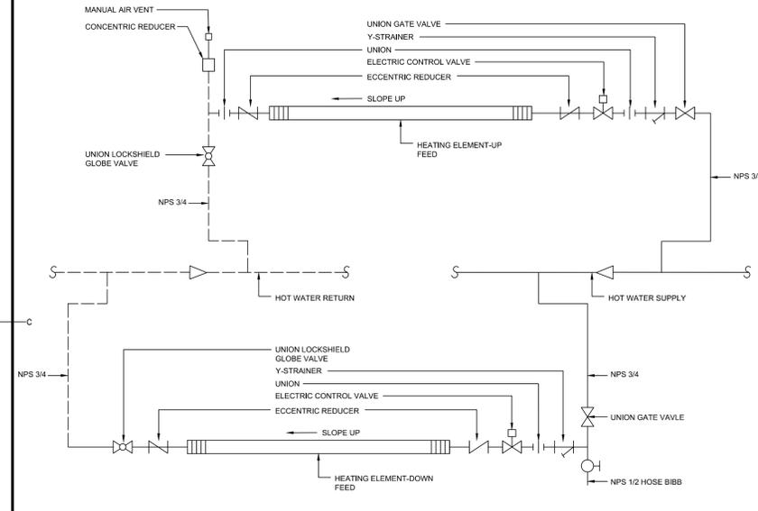
WALL FIN HOT WATER PIPING DETAIL - ONE ROW
