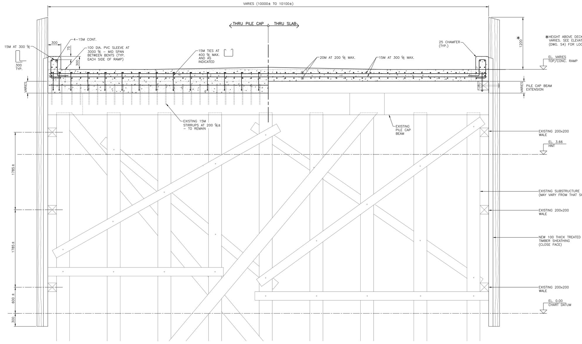
TYPICAL TRANSVERSE SECTION THRU STEM AT RAMP (Q 3/6)
