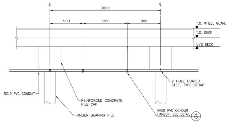
**ELEVATION - CONDUIT INSTALLATION UNDER CONCRETE PILE CAP WHARF, TYPICAL** (2 E2)
