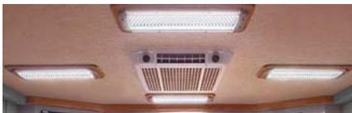
The lights must be activated by a three way switch placed on the interior right wall immediately inside the rear entry door and a second switch located on the forward wall immediately adjacent to the curb side work station.
