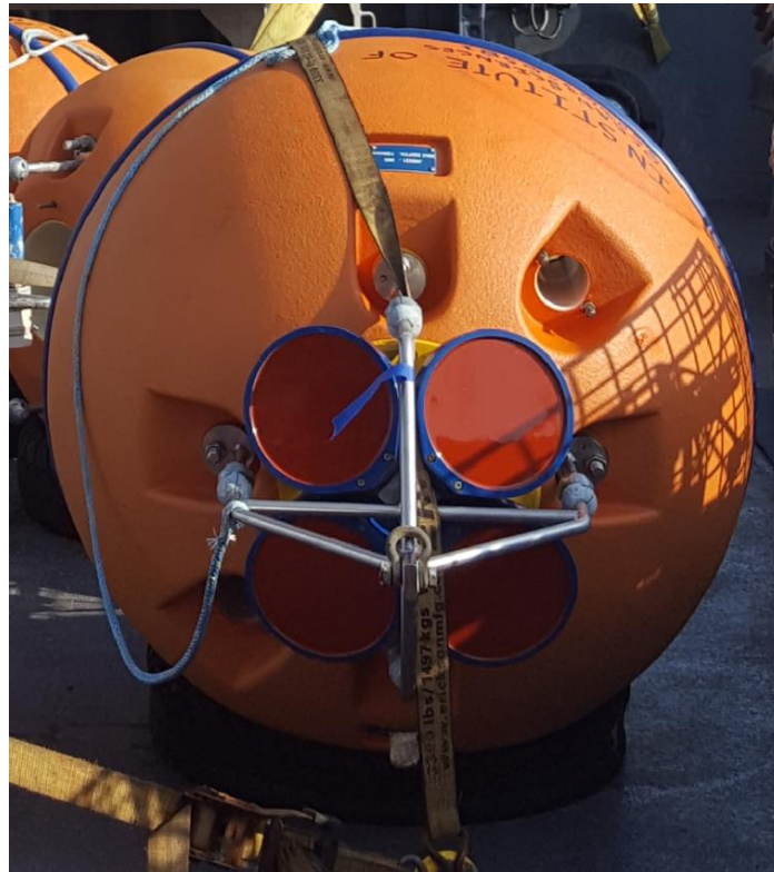
Figure 1 - A 44" float with a 75 kHz Long Ranger ADCP installed in the central instrument well. The secondary instrument well for the Seabird Microcat, and the associated 3/8"-NC titanium mounting studs, can be seen just above and to the right of the ADCP, and the well for the Iridium beacon can be seen to the lower left of the float. The four-beam symmetry of the mooring frame ensures that it does not obstruct the acoustic beams of the ADCP.
