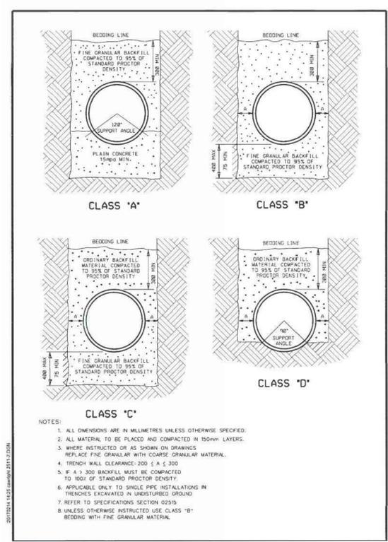
**STANDARD TRENCH BEDDING FOR CIRCULAR PIPES**
