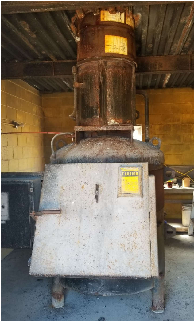
Figure 3: Existing Sable Island NPR incinerator
