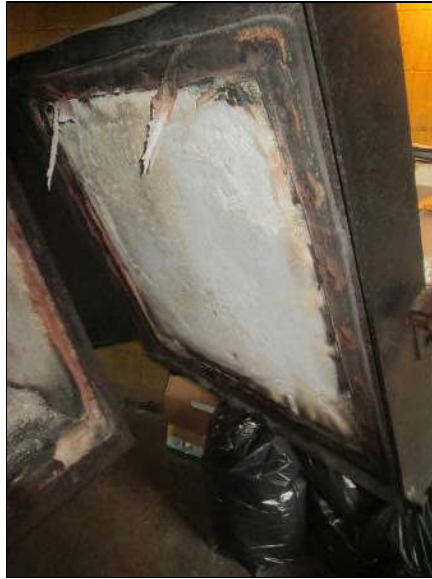
Photograph 1 – Asbestos-containing incinerator door gasket.
