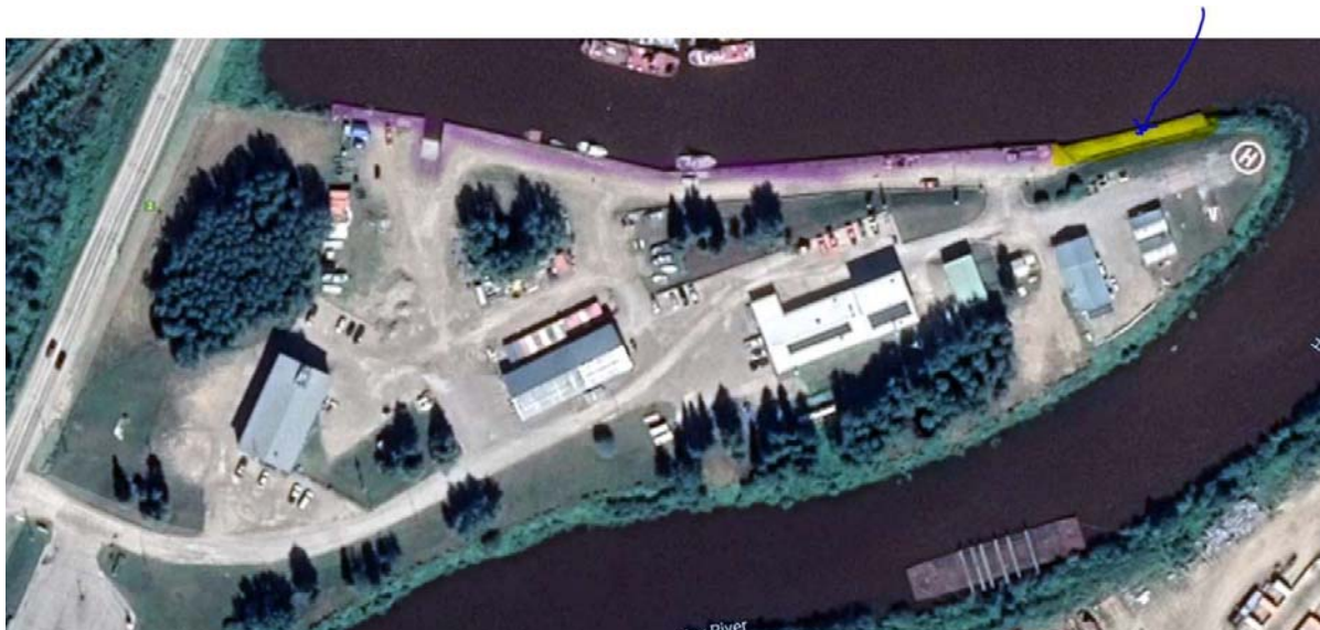
Photo 3: Sheet Pile Wharf (Purple to remain, yellow to be repaired)
