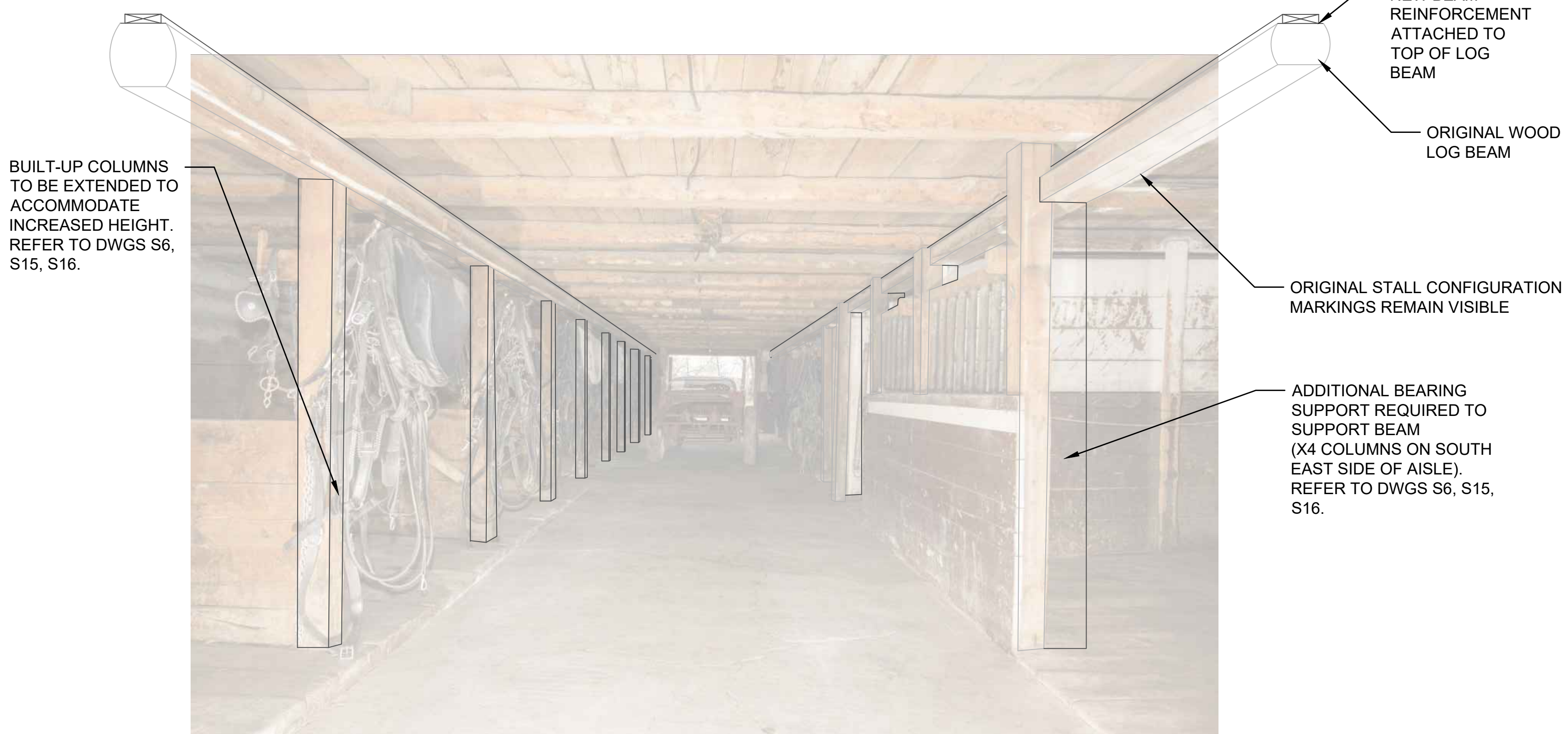
4 PERSPECTIVE OF NEW REINFORCEMENT ABOVE BEAM S8 NTS
