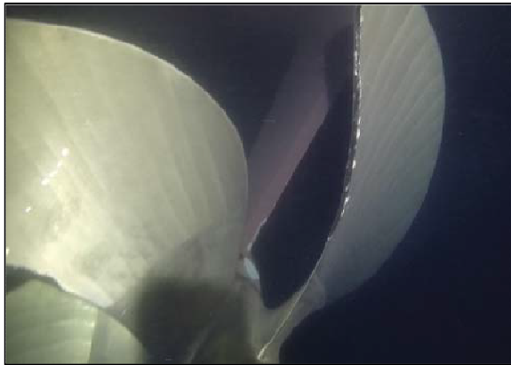
Anti-singing edge Photo Cred: Subsea Solutions
