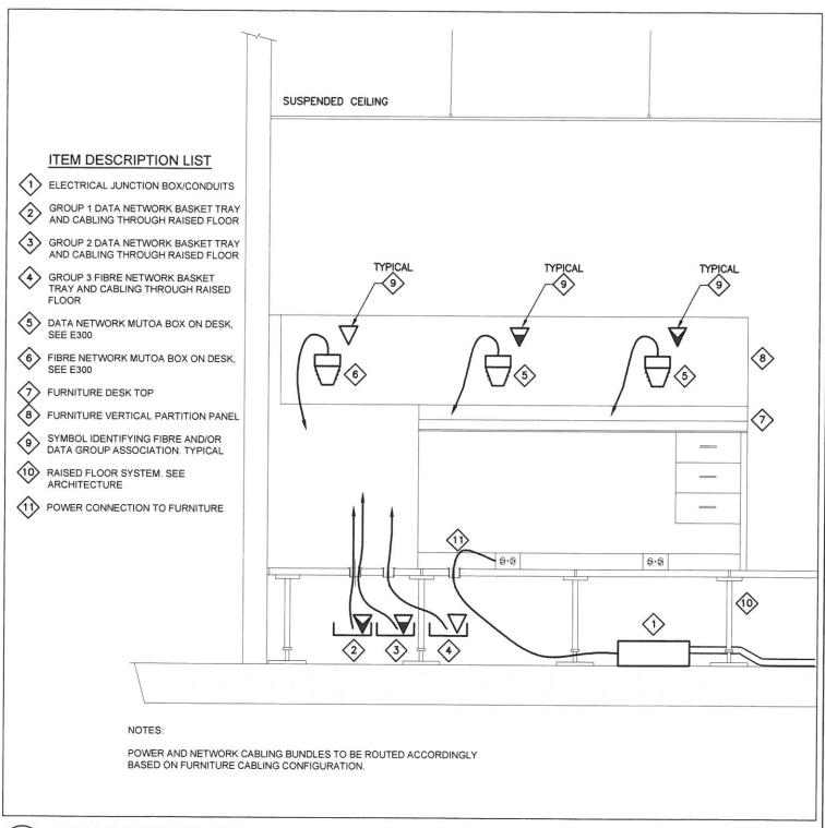
TYPICAL WORKSTATION DATA/FIBRE NETWORK CABLING DETAIL
