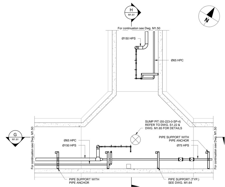
**2 MECHANICAL PIPING PLAN @ NTBU43+198 (BOTTOM Lvl)**
