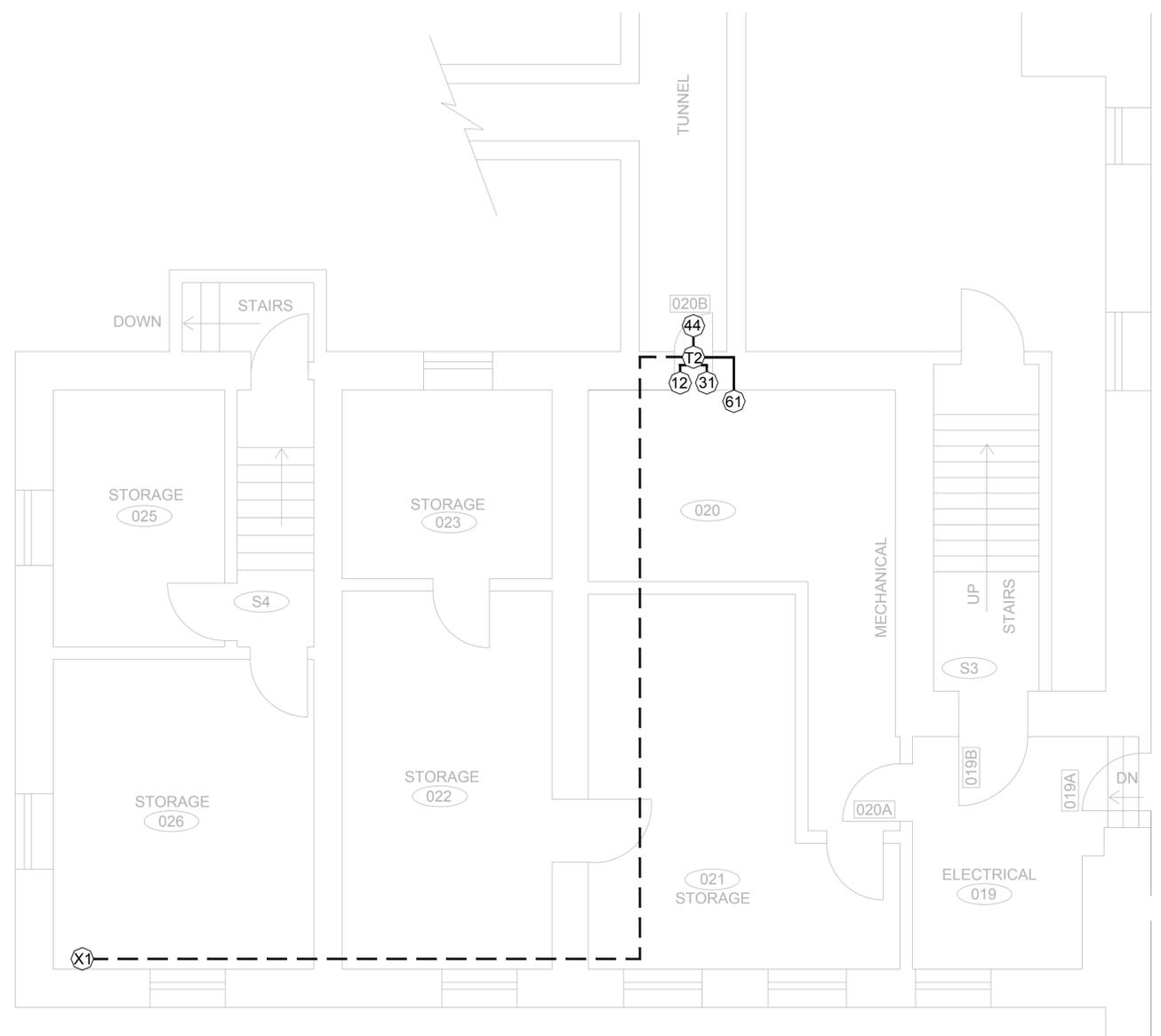
**1 | TBU 01 - DOOR 017 SECURITY SYSTEM PLAN - PTSS BASEMENT FLOOR**
