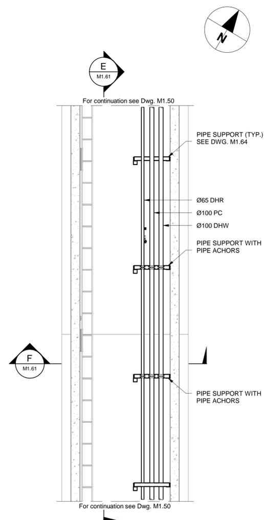
**1 MECHANICAL PIPING PLAN @ NTBU43+120 (TOP Lvl)**
