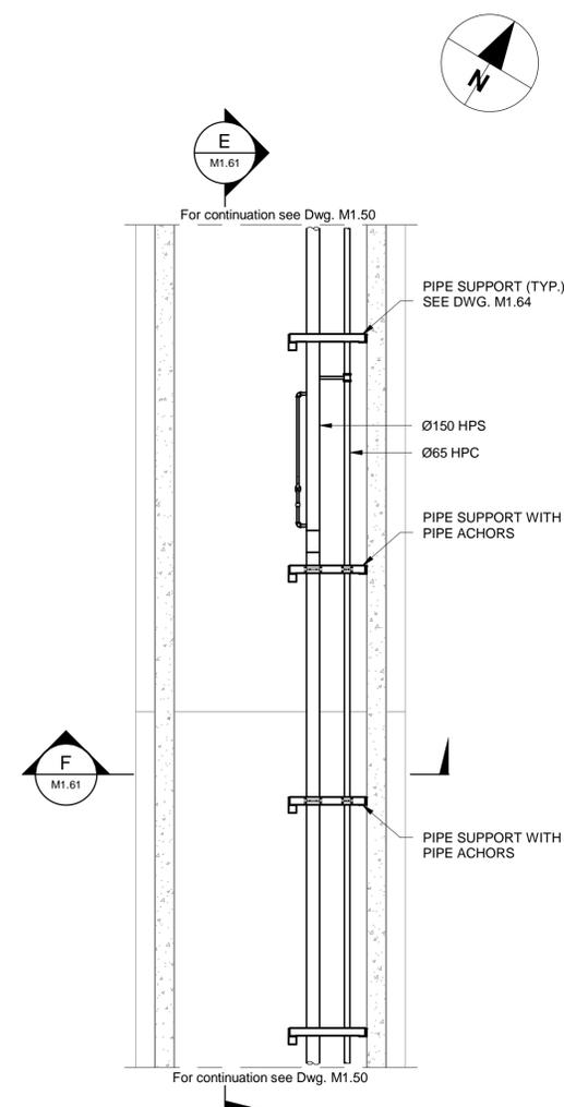
**2 MECHANICAL PIPING PLAN @ NTBU43+120 (BOTTOM Lvl)**
