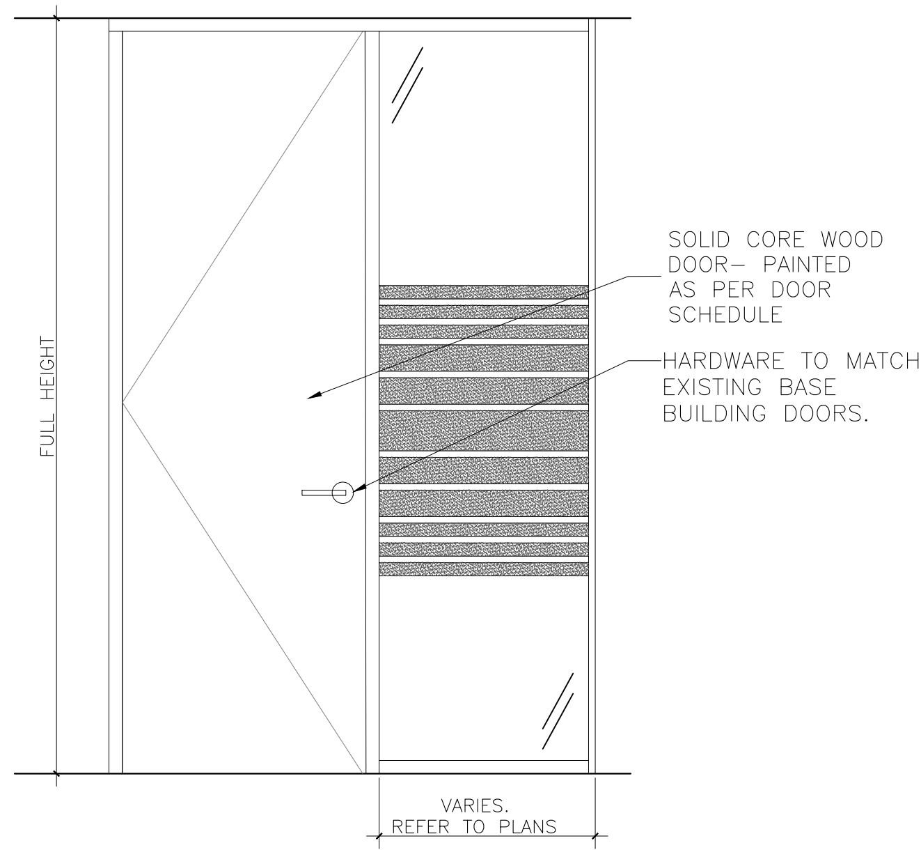
01 DOOR AND FRAME TYPE A (DEMOUNTABLE SYSTEM) ID 09 SCALE 1:20
