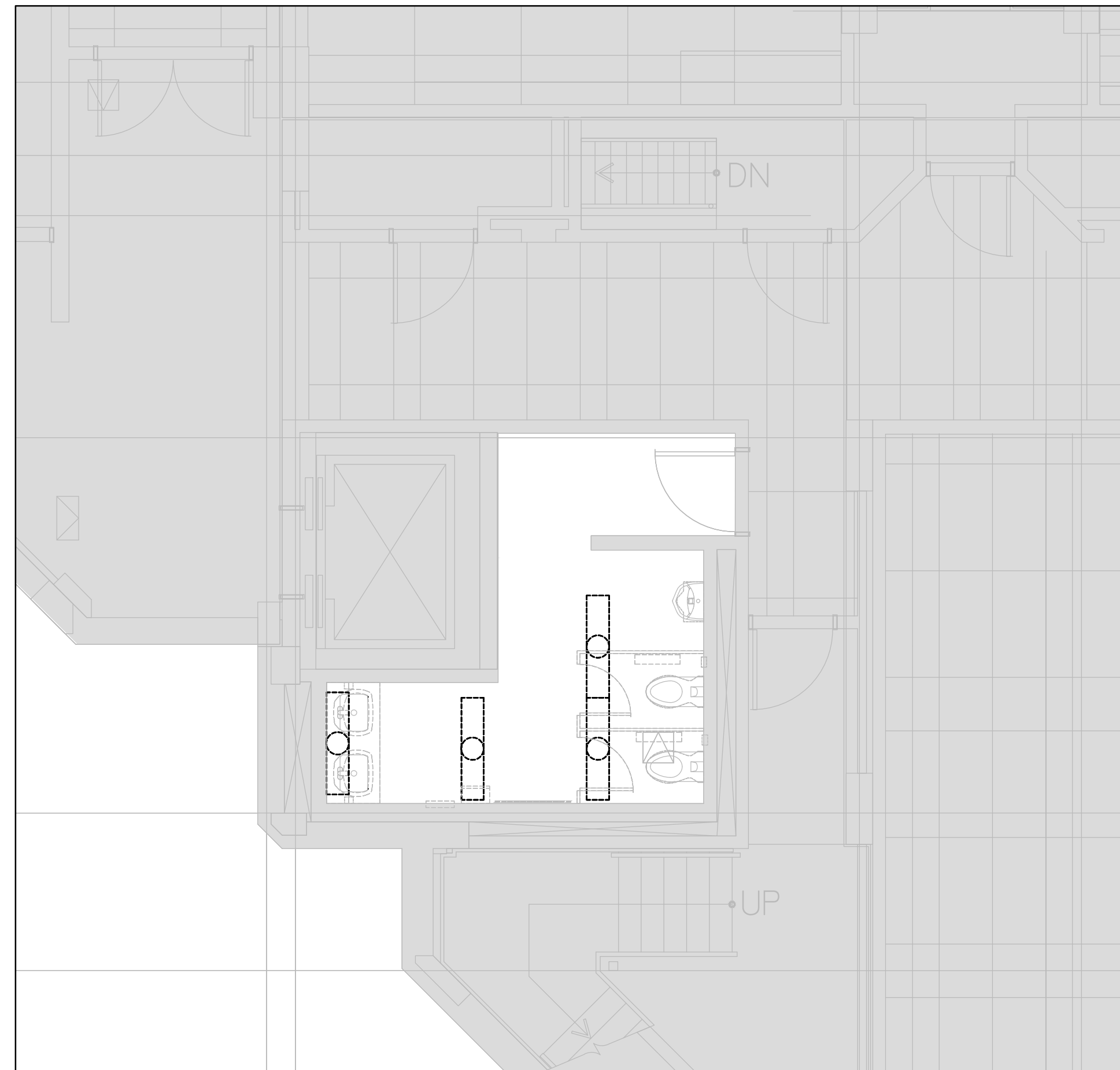
2 CEILING DEMO PL. - E WING -TYP. MEN'S WASHRM - TYPE D - SCALE - 1:50
