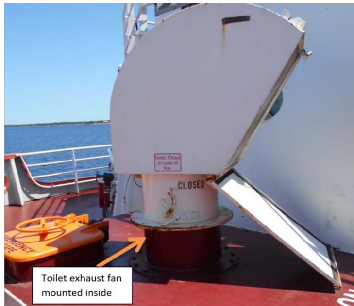
Figure 22: Photograph of in-situ toilet Exhaust axial fans
