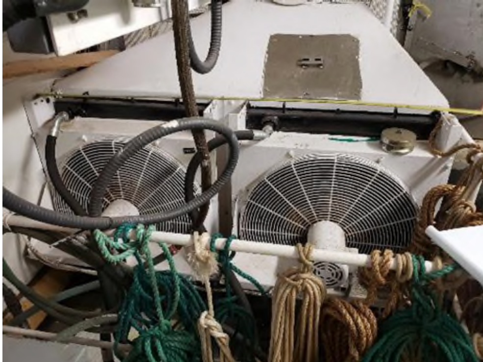
Photograph 3: View of Oil Coolers be to replaced and Air Intake
