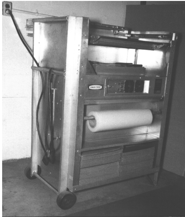
Figure 14-30 Skin Packaging Machine Figure 14-30 Machine pour emballage moulant
