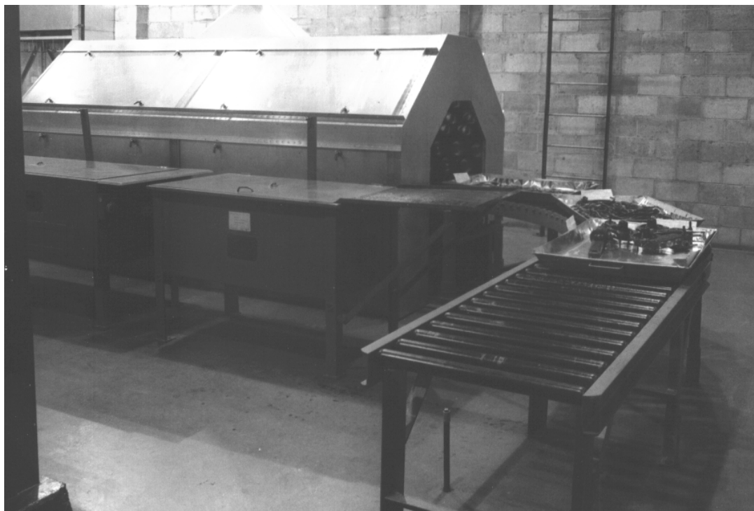
Figure 14-35 Infra-Red Drying Oven Figure 14-35 Séchoir-tunnel à infrarouge
