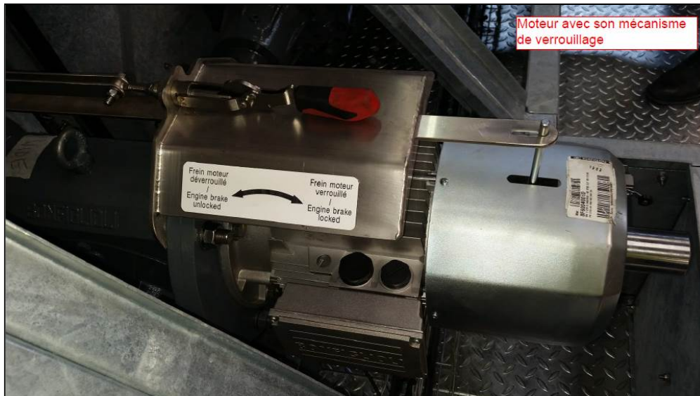
Figure 22: Latchford Dam gate hoist. Gear reducer (at left) and motor. Photo taken in factory.
