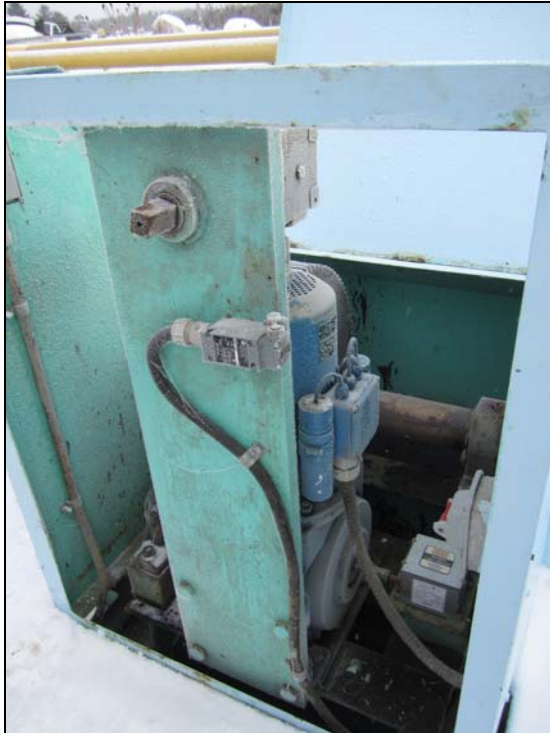
Figure 6: Portage Dam, detail of hoist enclosure with front removed.
