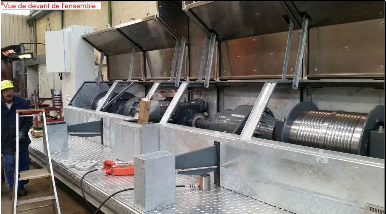
Figure 21: Latchford Dam gate hoist under construction in factory.
