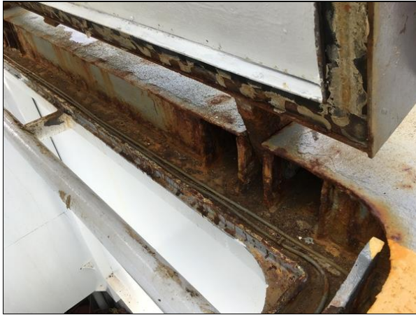
Figure 19: Condition of coaming, compression bar & Rubber Packing. One can see remaining of neoprene glue on top of rubber packing face.
