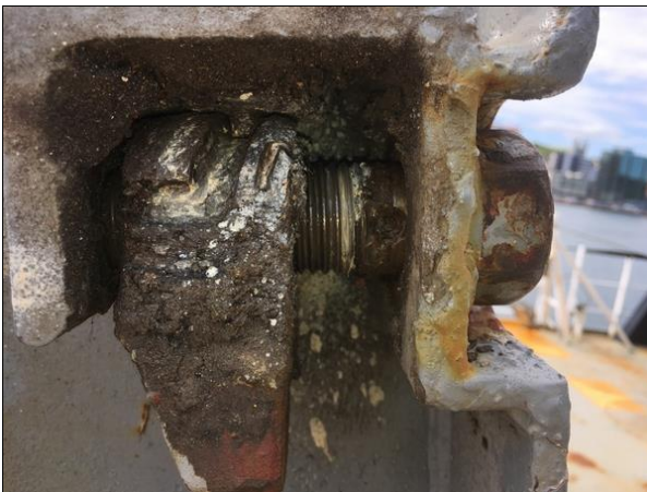
Figure 17: Condition of flush deck cleats. This one has a missing Spring Pin
