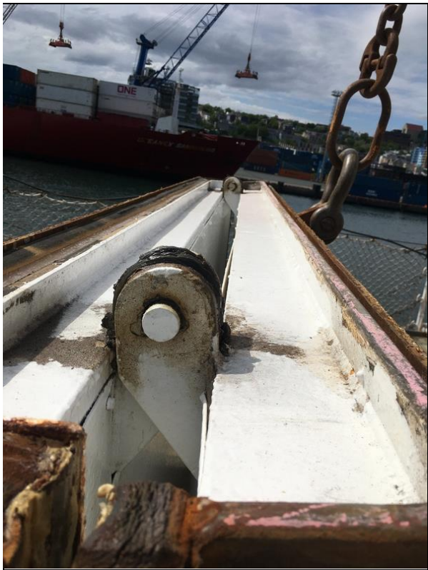
Figure 12: Intermediate Hinges on PS HC
