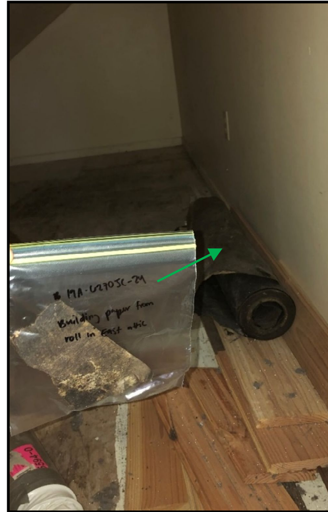
Sample 19A-6270JC-23 of building paper from the upper level top of staircase behind wood siding was 'None Detected' for asbestos (left). Sample 19A-6270-JC-24 stored roll of building paper within the side attic was 'None Detected' for asbestos (right).
