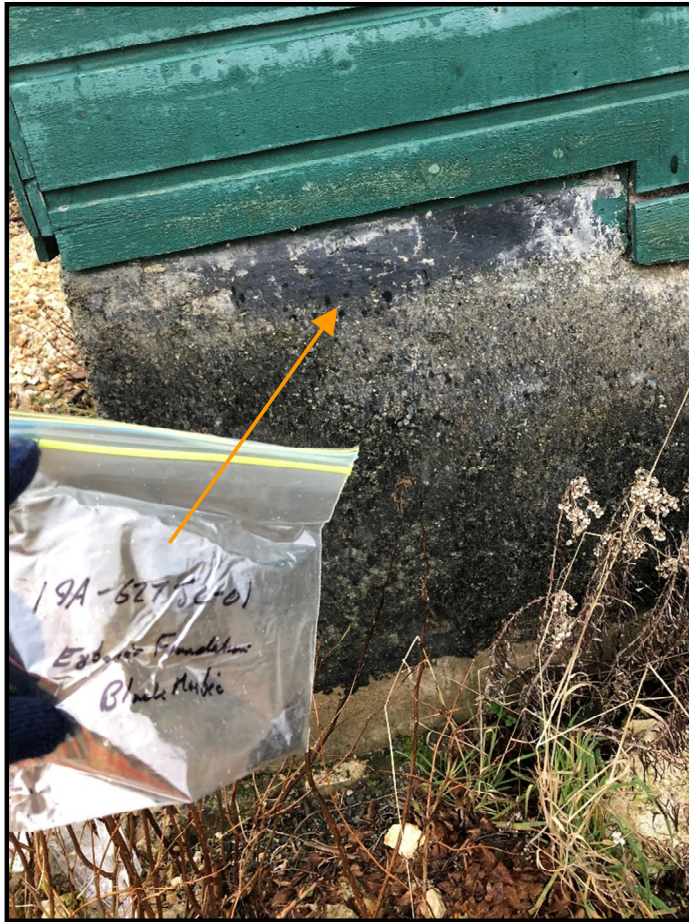
Sample 19A-6270JC-01 black mastic on exterior perimeter foundation (PC 0.25% Chrysotile) (left).
