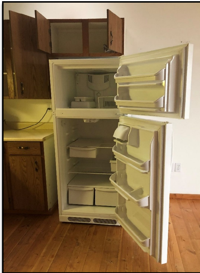
A domestic style refrigerator was observed in the kitchen which may contain ozone depleting substances (ODS).
