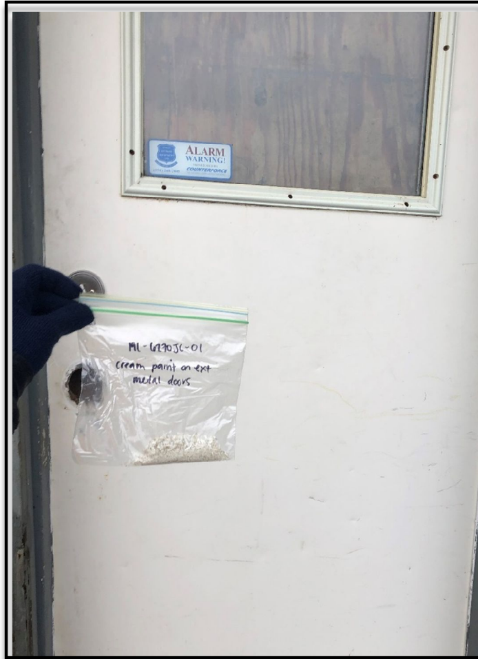
Cream paint sample 19L-6270JC-01 applied to the exterior metal doors with lead concentration: 0.041 wt% (410 ppm).
