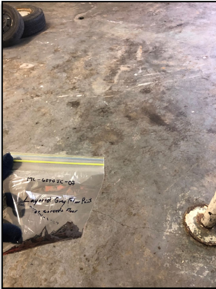
Layered grey paint sample 19L-6270JC-07 applied to the warehouse concrete floor with lead concentration: 0.011 wt% (110 ppm).
