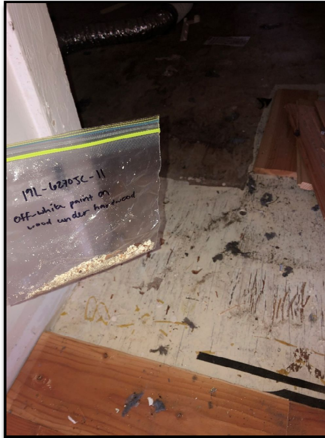
Off-white paint sample 19L-6270JC-11 applied to the upper residence sub-floor at the entrance to the side attic with lead concentration: <math><0.0080\text{ wt\%}</math> (<math><80\text{ ppm}</math>).
