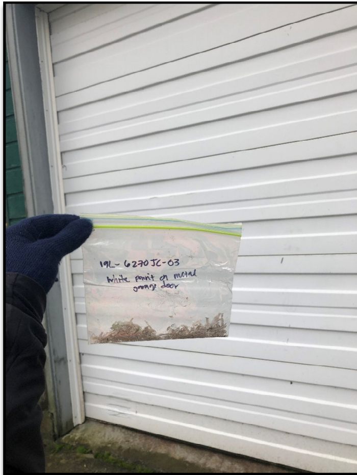
White paint sample 19L-6270JC-03 applied to the exterior of the roll-up metal door with lead concentration: <math><0.0083\text{ wt\%}</math> (<math><83\text{ ppm}</math>).
