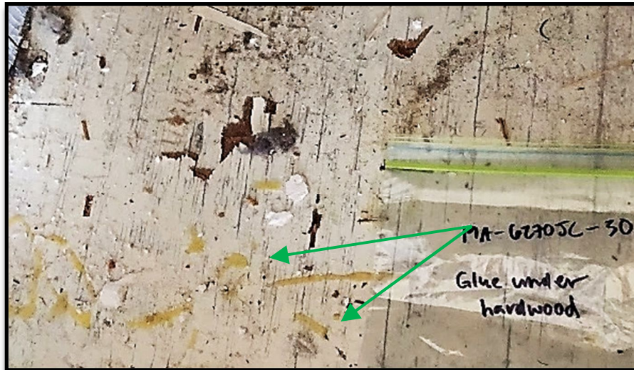
Sample 19A-6270-JC-30 glue on the subfloor under plank flooring at the entrance to the side attic was 'None Detected' for asbestos (left). Sample 19A-6270-JC-31 building paper under plank flooring at the entrance to the side attic was 'None Detected' for asbestos (right).
