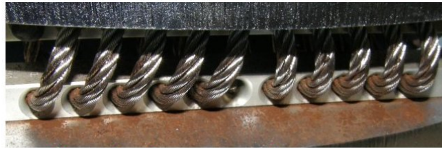
Rust from wire rope
