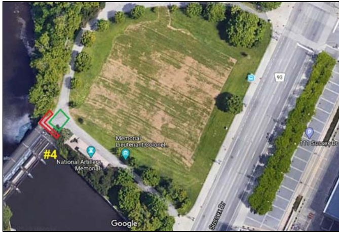
Figure 10: Crane location for Sluice #4. Crane may park in green area. Outriggers must avoid red area.
