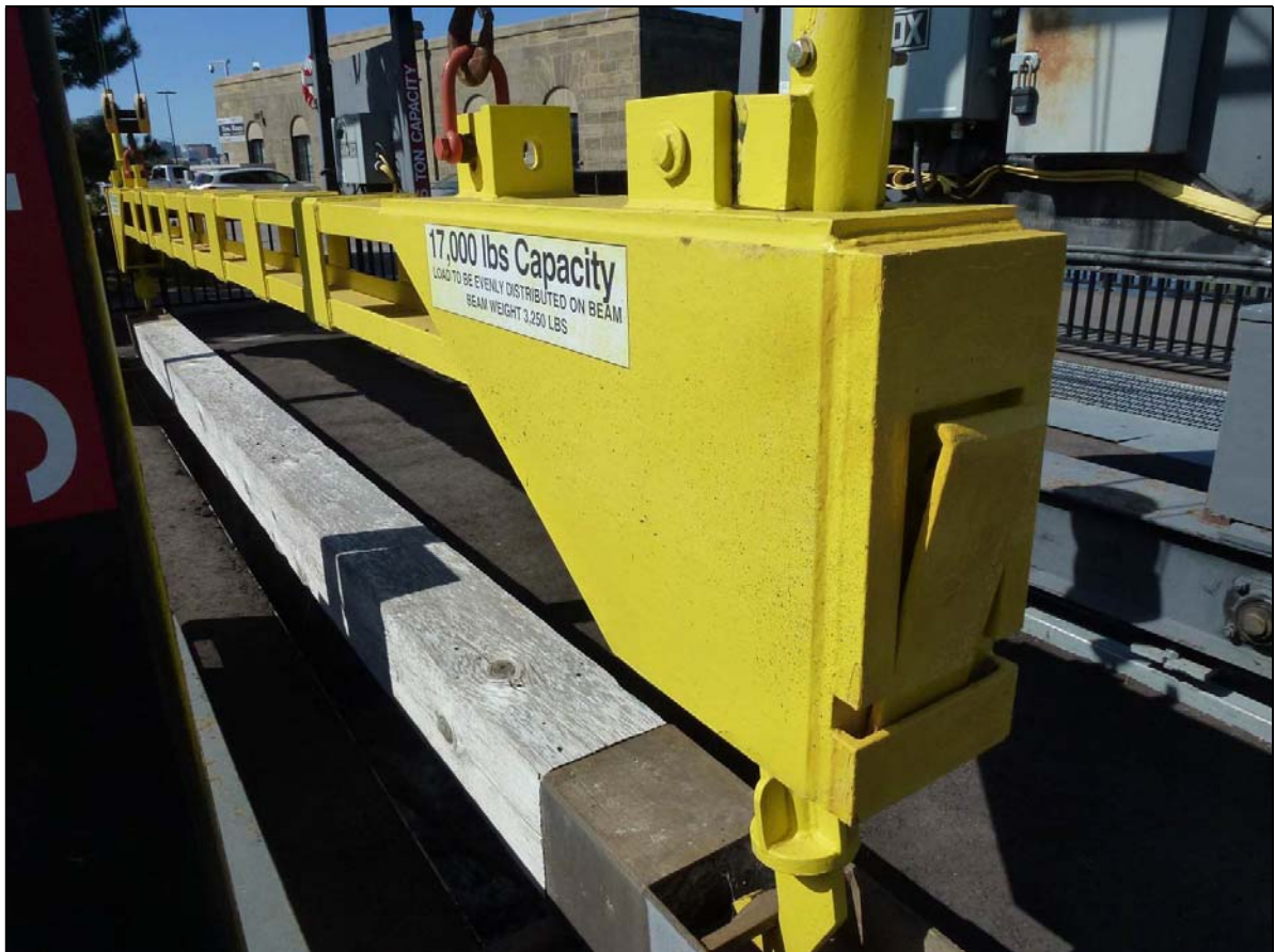
Figure 5: Spreader beam for stoplogs.
