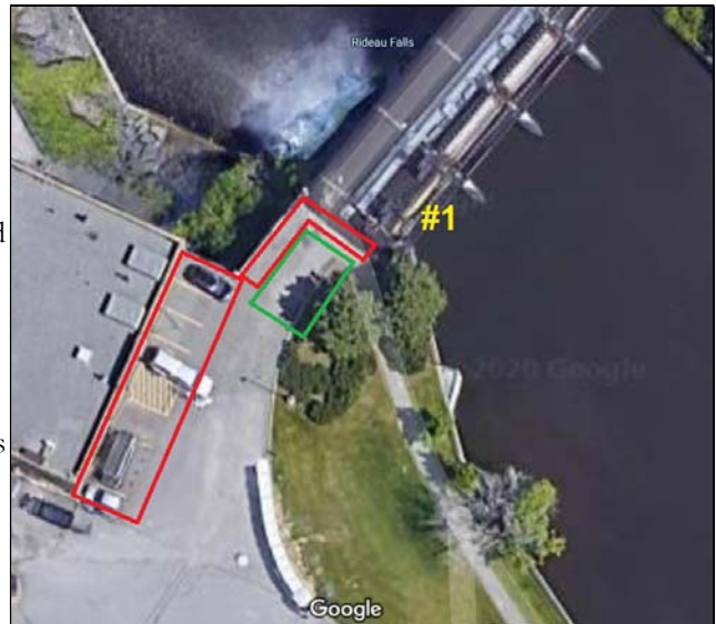
Figure 8: Crane parking for access to Sluice #1 shown in green. Areas to avoid are shown in red.
